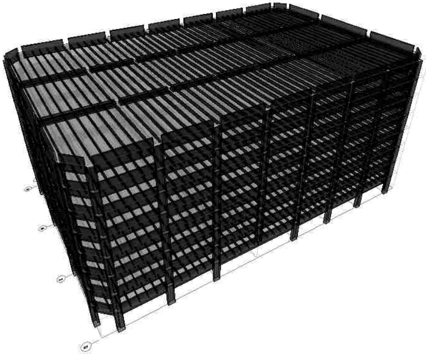
Figure 5-1: 3-D extruded view of the model simulated in ETABS
