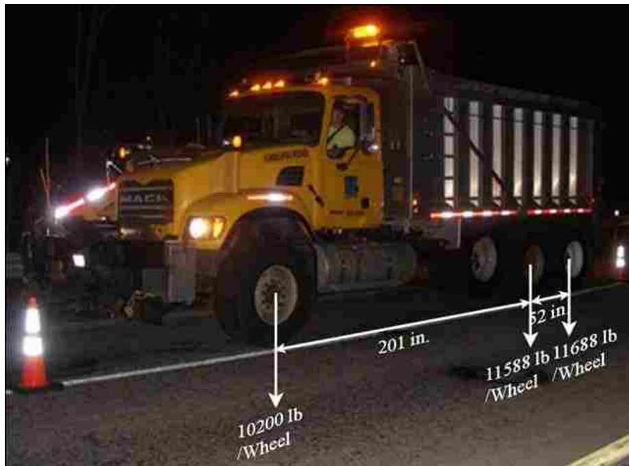
Figure 2-10: Test truck used during controlled load tests
