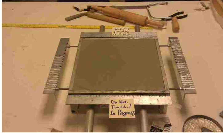
Figure 1.1- Testing Tray Packed with clay and Fiber Optic grid
