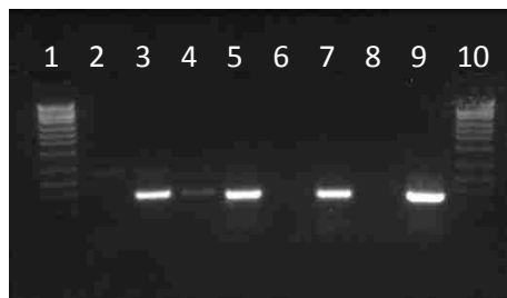
Figure C-2. UV photograph of 4/26/11 Queen Lane water filter samples after 60 minutes of gel electrophoresis in a 1.4% agarose gel. From left to right, the lanes are as follows (1) 1 kilobase pair ladder, (2) 4/26/11 QLA Sample, (3) 4/26/11 QLA Sample, (4) 4/26/11 QLB Sample, (5) IMS positive control, (6) IMS negative control, (7) DNA extraction positive control, (8) DNA extraction negative control, (9) primary PCR positive control, and (10) an additional 1kbp ladder (primary PCR negative control, secondary PCR positive control, and secondary PCR negative control are not shown). The QLA sample was processed by DNA extraction and nested PCR in duplicate,
