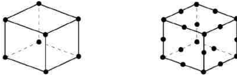
Figure 3.13: Representations of the two types of p-convergence methods used in this study. The 8 node linear heat transfer element shown on the left and the 20-node quadratic heat transfer element shown on the right.
