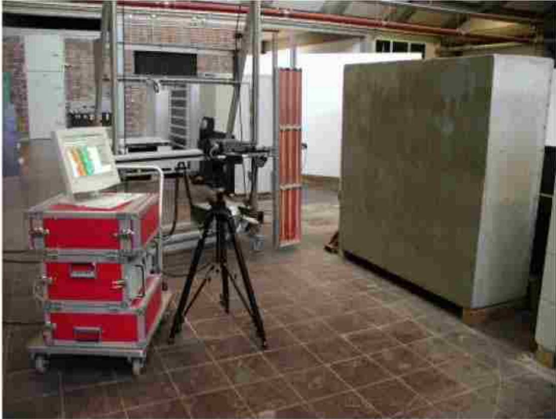
Figure 3.2: Experimental Setup of BAM experiment, including the concrete block specimen, the radiator, the infrared thermography camera and the computer unit (Wiggenhauser, Hille and Cziesieki 2004)
