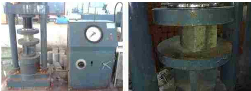
Figure 5 Experimental set up for testing of cubes for compressive strength [11]
