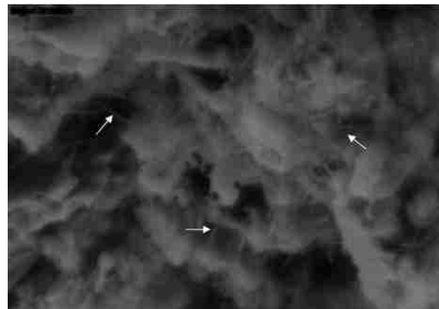
Figure 23. SEM image of 0.03% CNT/cement specimen [8]
