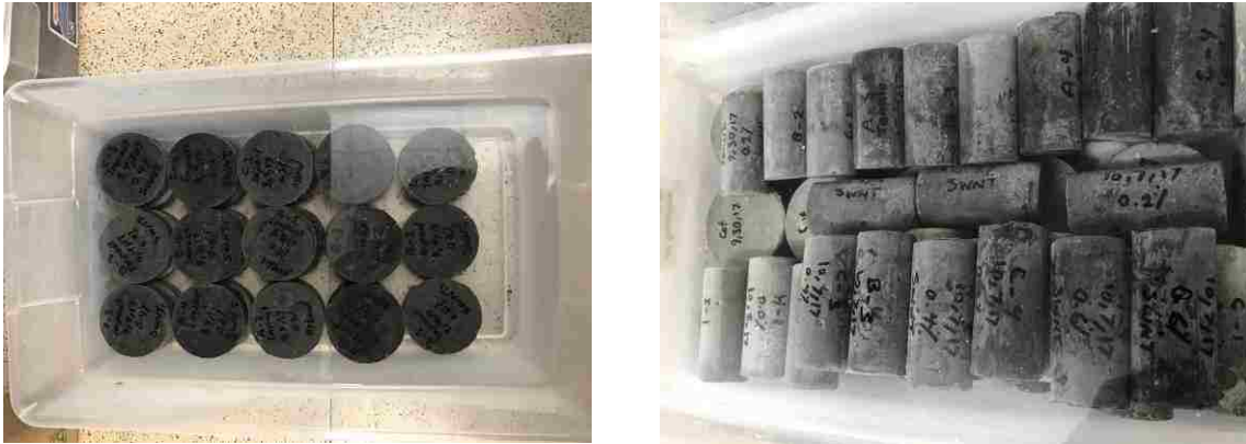
Figure 53. Impact and tensile cementitious nanocomposite specimen curing
