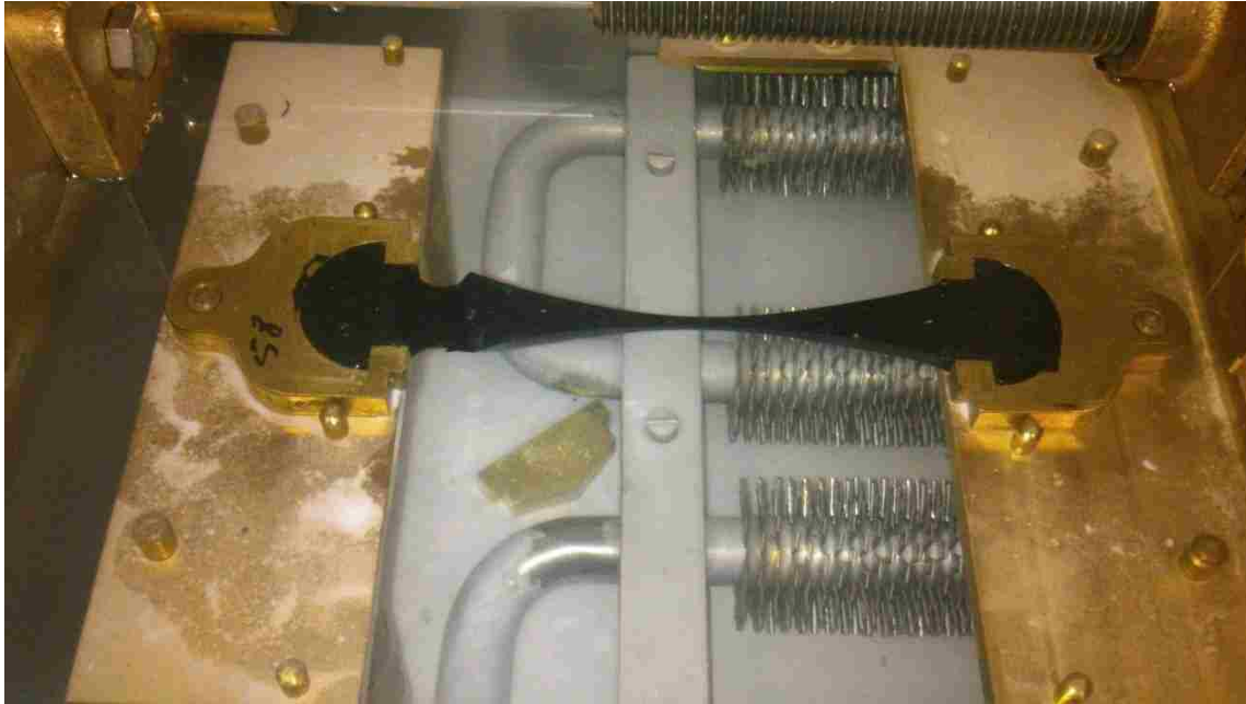
Figure 37. Ductility of binder PG 58-28 mixed with CRM
