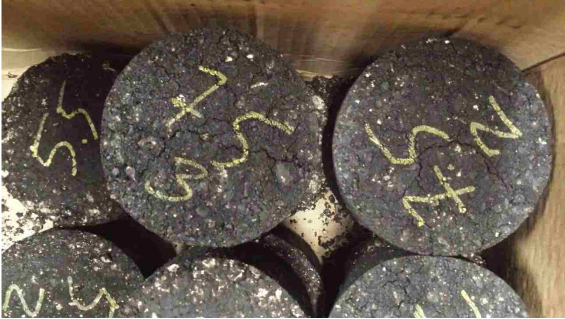
Figure 65. Pack of samples leaded to defective wave propagation
