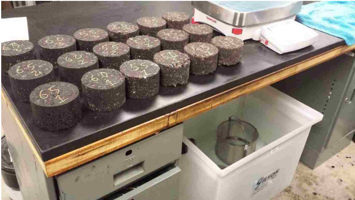
Figure 41. Pack of compacted samples next to density measuring tool
