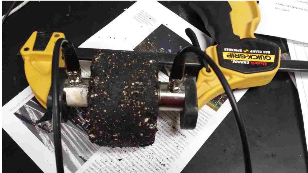
Figure 48. Sample fixed between two transducers
