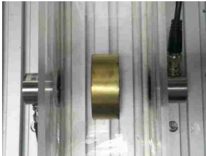
Figure 23. Transducer during the measurement, a: contact, b: immersion
