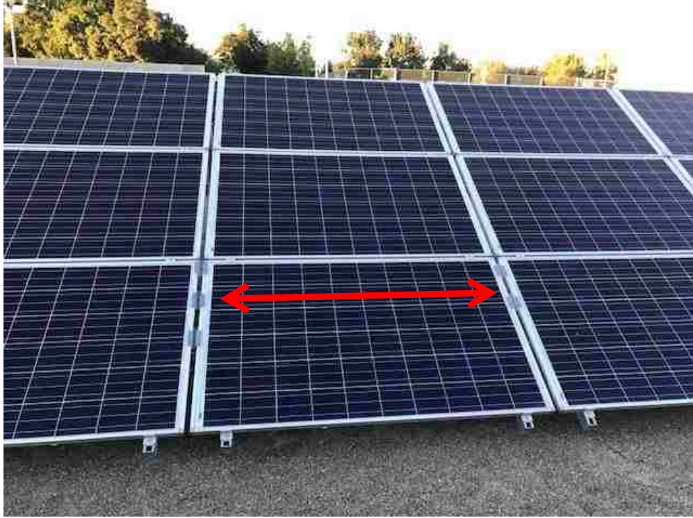
Figure 9. Tempered glass samples fixed to the solar panels to verify the amount of dust accumulated per cleaning, and the efficiency of cleaning
