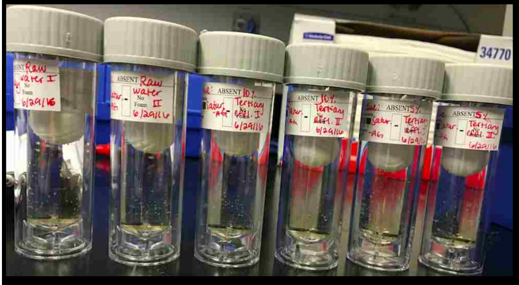
Figure 30. Utility 2. From left to right, S 2 and duplicate, 10% Wt 2 / S 2 and duplicate, 5% Wt 2 / S 2 and duplicate. Foam around and under the ball was a positive test for denitrifying bacteria.
