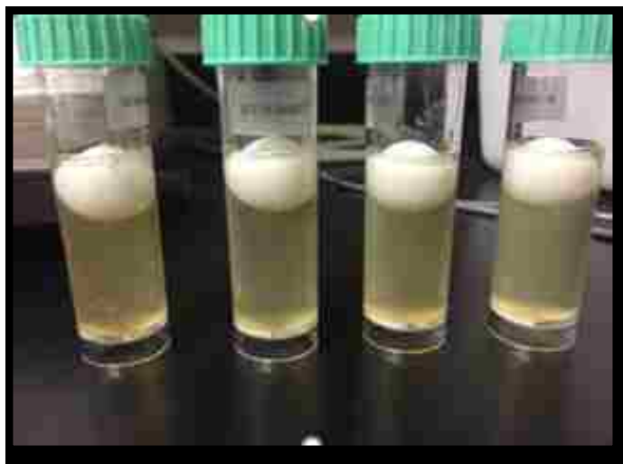
Figure 29. Utility 2. From left to right, 10% Wb 2 /S 2 and duplicate, 50% Wb 2 /S 2 and duplicate. Cloudy solution and dense slime growth at base was a positive test for the presence of slime forming bacteria.
