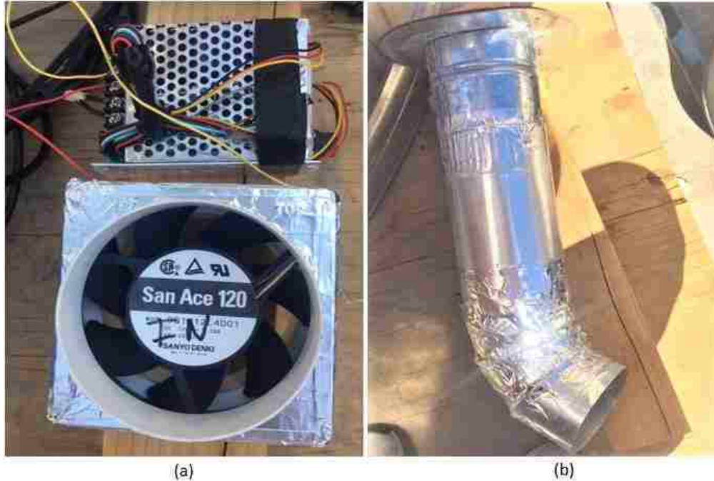
Figure 3-3 Blower components, which include a: (a) 4-in fan with a speed controller and (b) 4-in duct with a 45° angle bend on the bottom.
