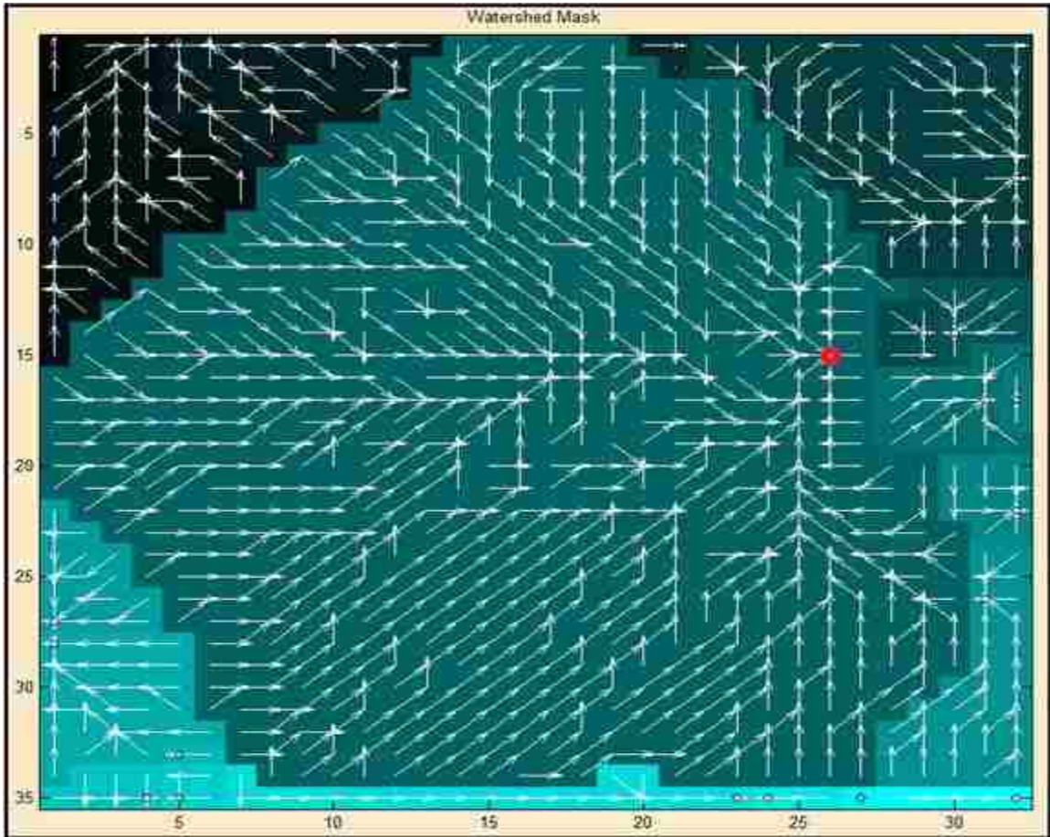
Figure 5.2-3: Catchment areas within the UNLV Parking-lots study area predicted by the model. Pixel with red dot represents the pour-point pixel.
