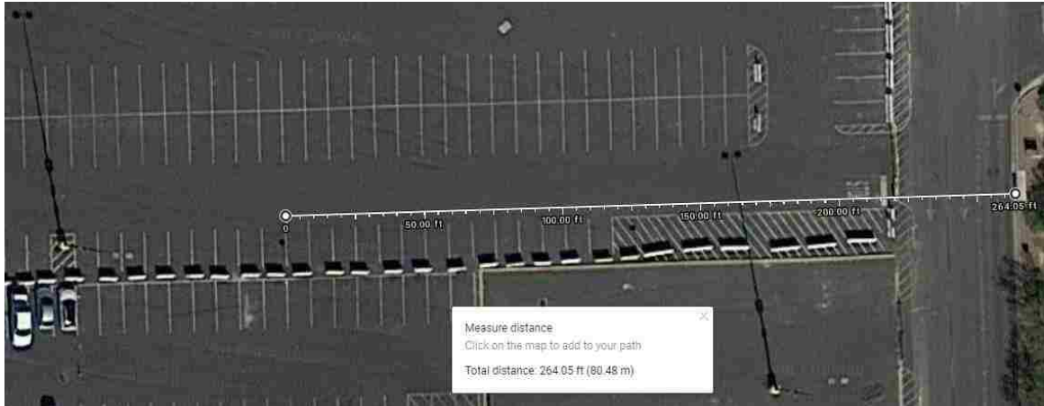
Figure 5.2.4-3: Distance from drainage inlet to the actual maximum extent of flooding towards the West end as measured in Google-Map.
