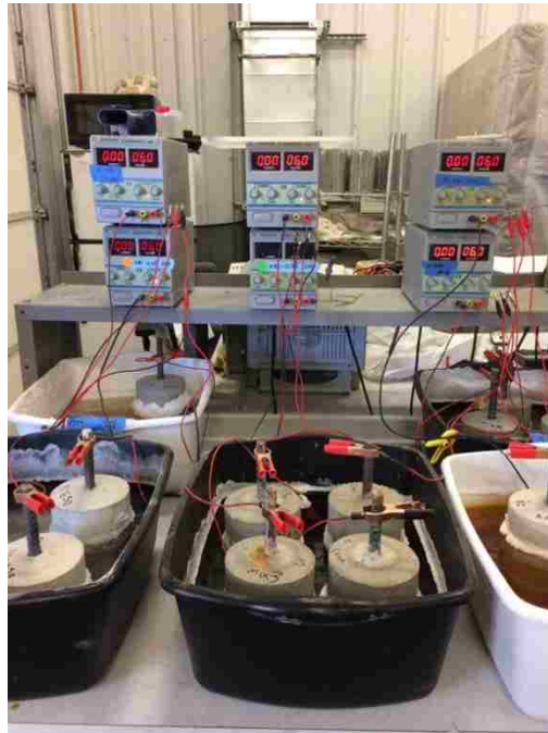
Figure 2. 8: Accelerated Corrosion Setup
