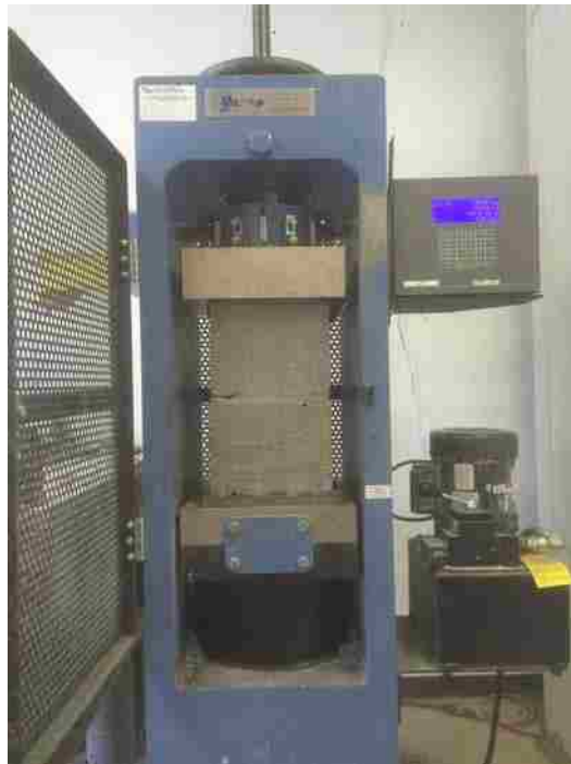
Figure 6- Example of Prism Testing in Compression Machine
