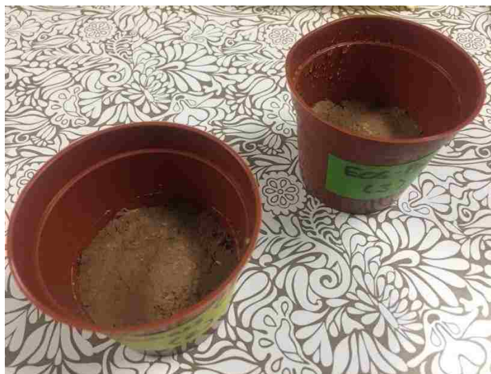
Figure 3-5: Two finished soil samples prepared for incubation at ambient conditions. The water visible on the pot is from spraying to prevent premature drying of the sample.
