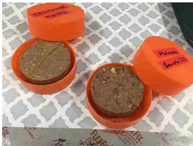
Figure 3-2: Finished soil samples placed in labelled Shelby tube end caps. These were wrapped in aluminum tape to prevent any air from reaching the samples, effectively sealing them completely. The lines in each sample indicate how much to take for contaminant analysis.
