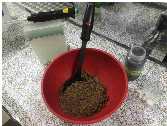
Figure 3-4: Soil being mixed with bacteria and nutrients for the advanced bioremediation sample preparation.
