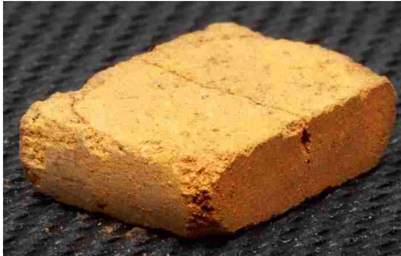
Figure 14: Processed Simulated Martian Soil Brick (Grush, 2017 [David Bailot])
