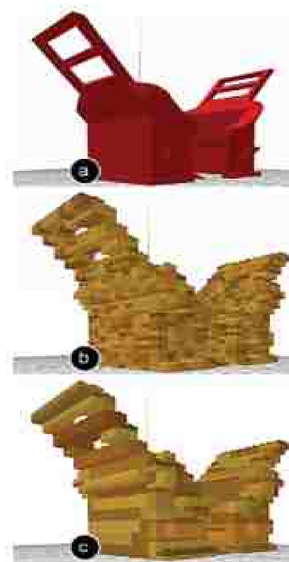
Figure 6: (a) Model Loaded into faBrickator, (b) Legofied into 1x1 Lego Pieces, (c) Layout Model (Mueller et. al., 2014)
