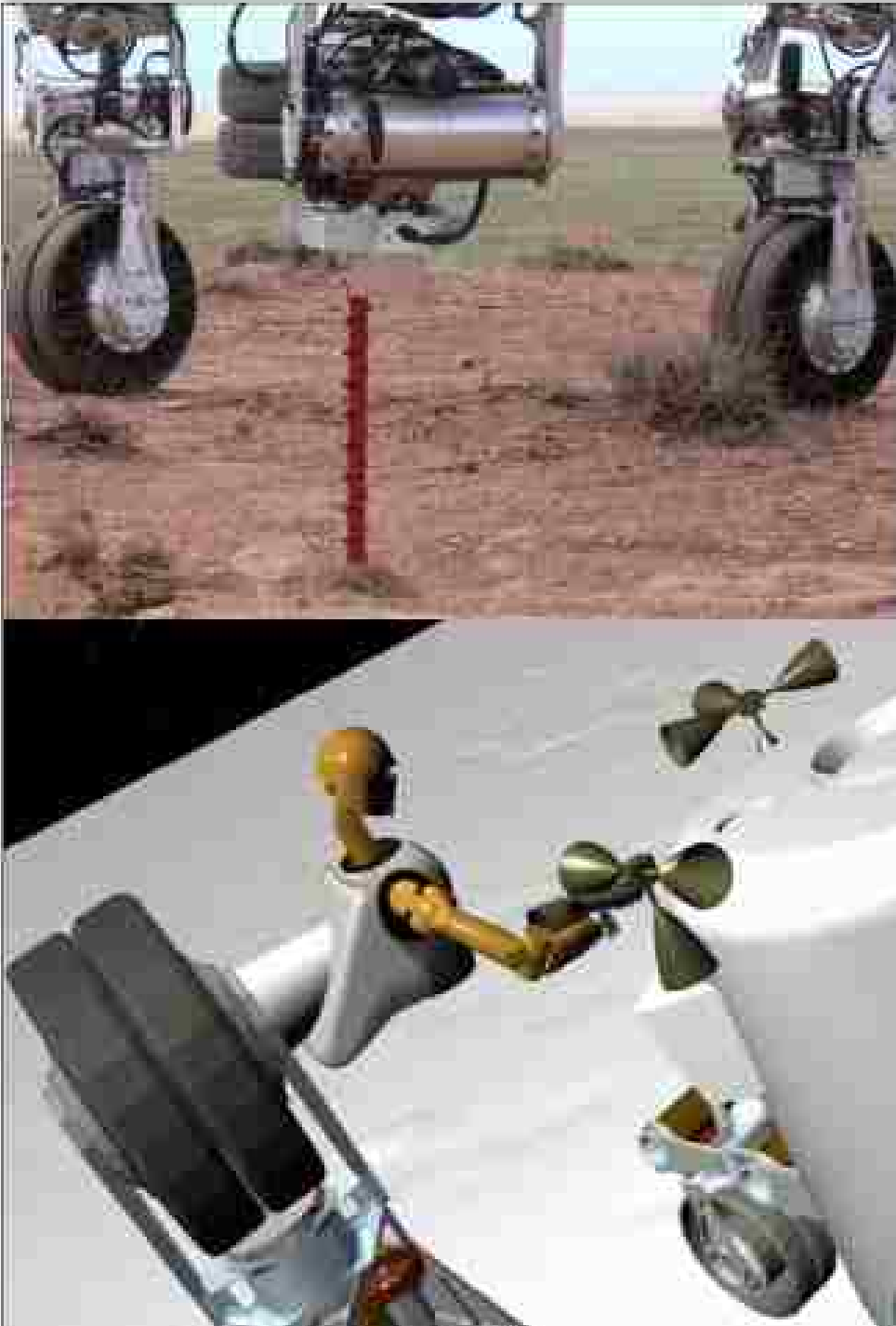
Top - ATHLETE drilling tool in natural terrain
