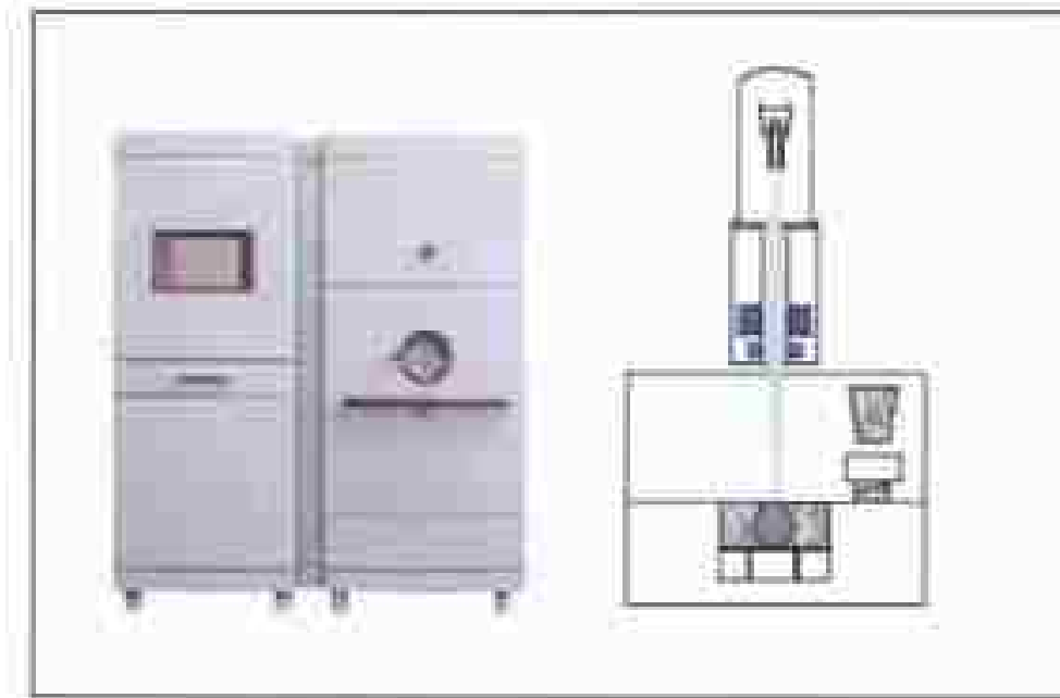
Figure 9: Arcam EBM Machine and Schematic (Howell et. al., 2007)
