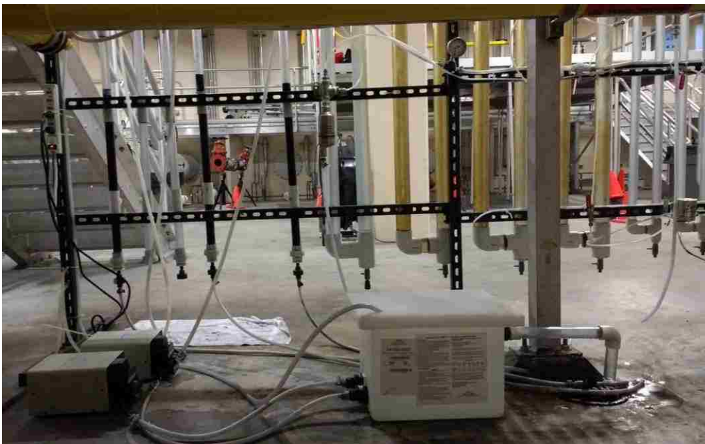
Figure 19. One liter per minute pilot-scale ozone-biofiltration system seen from the opposite side as in Figure 18. Peristaltic pumps (bottom left) to the biofilters and tank with ozonated water with no residual ozone.
