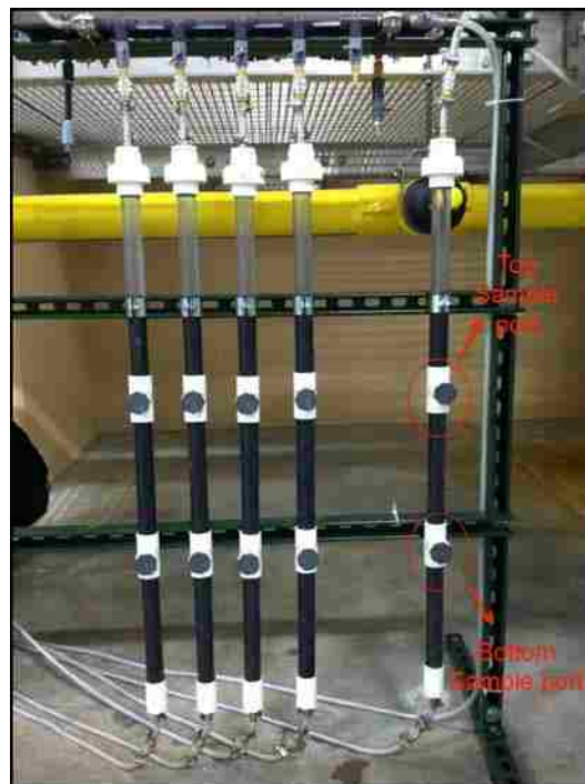
Figure 25 – Layout of biofilter and location of media sample ports
