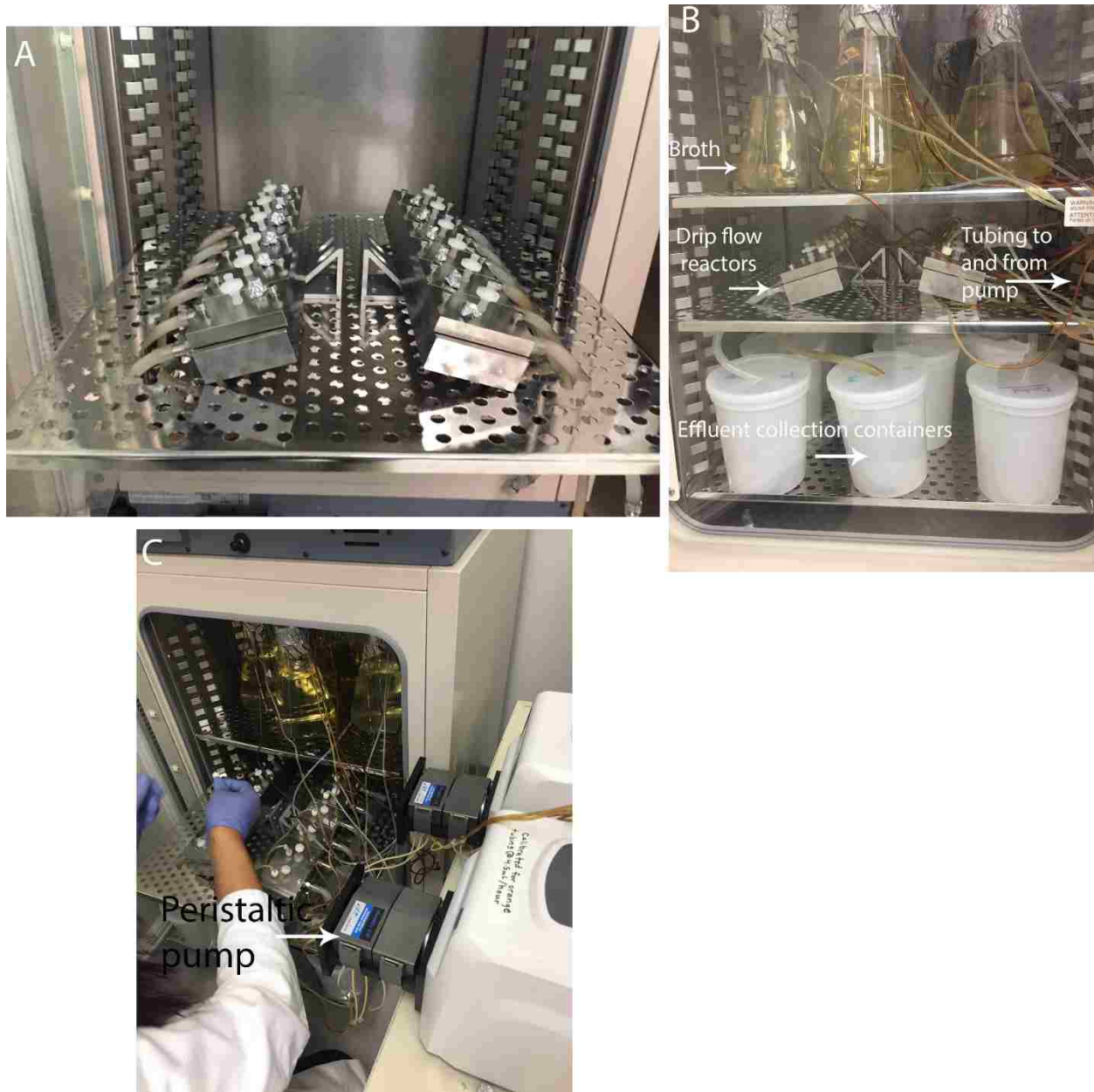
Figure 3.3: Setup of the modified drip flow reactors. (A) Two reactors could be used at a time in the standing incubator. (B) Broth was flowed through each tube using a series of tubing. The effluent ports allowed broth to drain. The system allowed for shear force, fluid and air exchange to occur. (C) Peristaltic pumps were used to flow broth through each chamber. Tubes were red through a pump head that rotated, creating flow.
