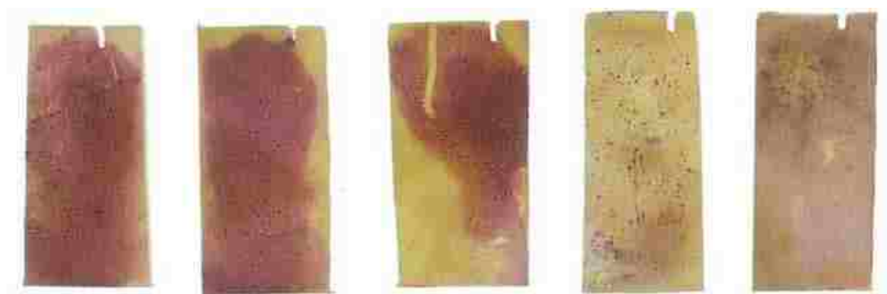
Figure 4.11: Gross photographic images of coupons that had CZ-99 and silver benzoate incorporated. As with controls, red/purple areas were indicative of ruthenium red that stained the biofilms.
