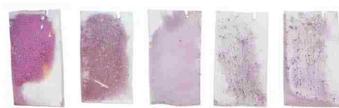
Figure 4.9: Gross photographic images of positive control coupons. Red/purple areas were indicative of ruthenium red that stained the biofilms that were present. The pattern of broth flow was also highlighted by the stain. Note the speckled appearance in many regions. These were plumes of biofilms, as verified by the SEM images provided below.
