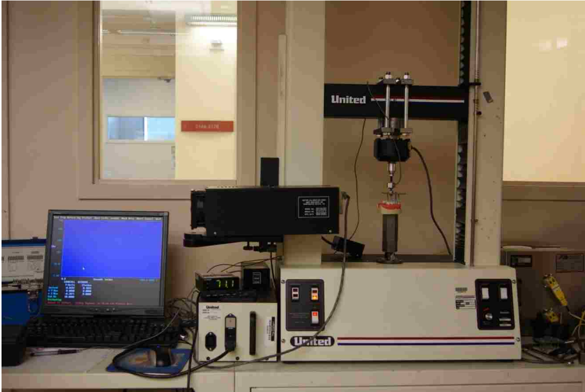
Figure 3.4- Experimental set up using Universal Testing Machine
