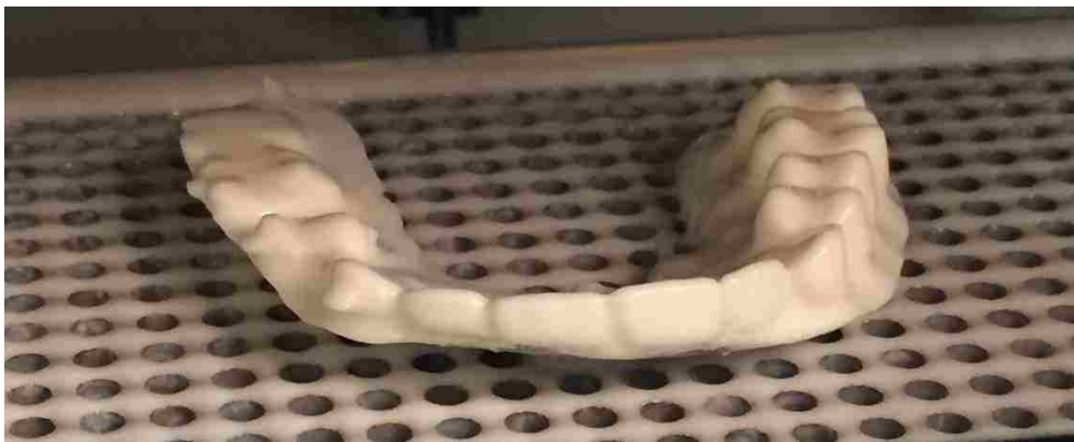
Figure 5-2 Model warpage on left side
