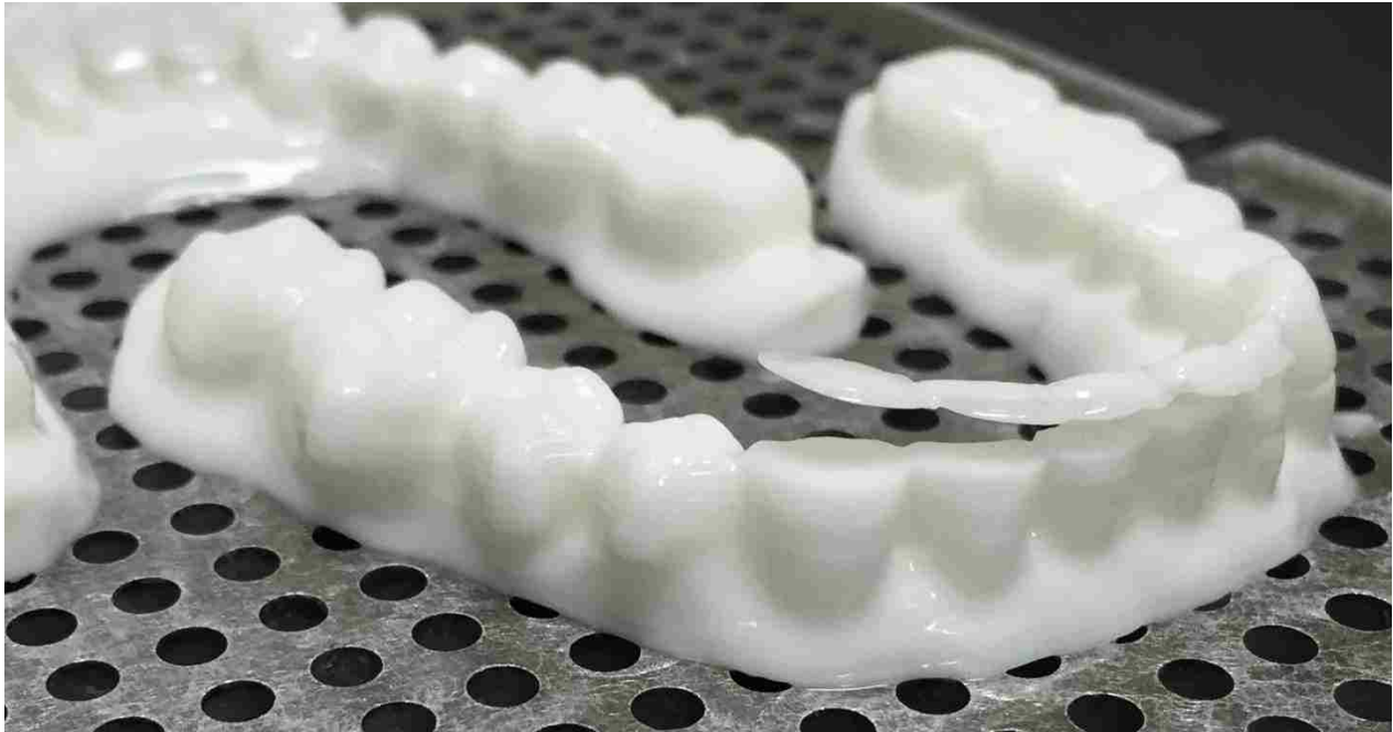
Figure 5-3 Omitted layer from object slicing error
