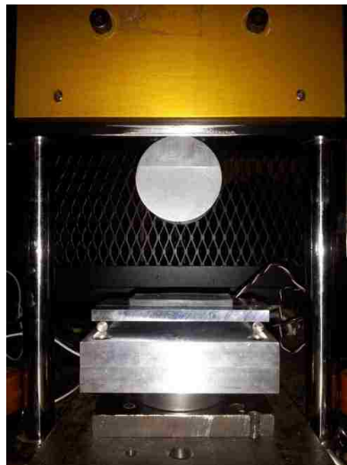
Figure 9. Simply supported beam testing method
