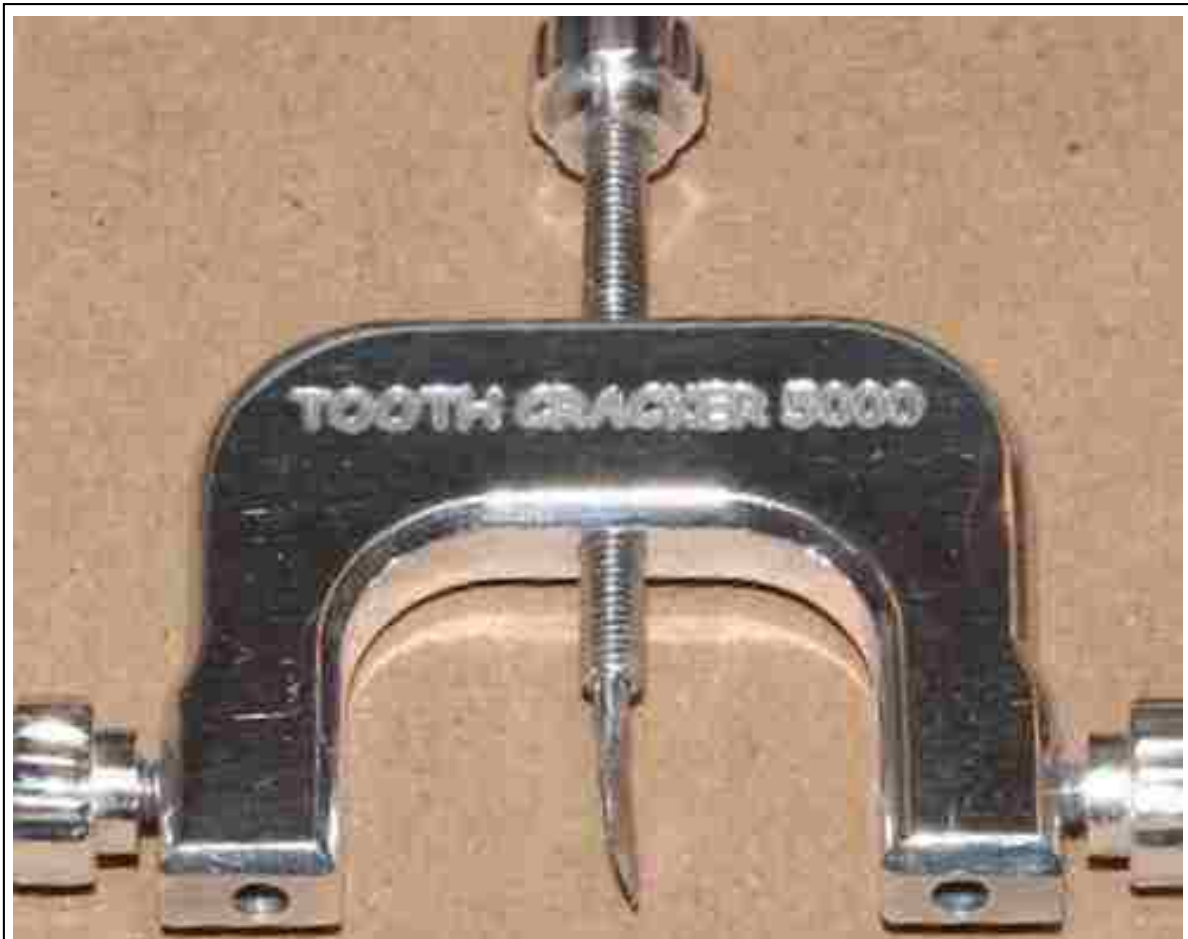
Figure 15. Splitting Blade (bottom Center) and Splitting Knob attached to threads (Top Center)
