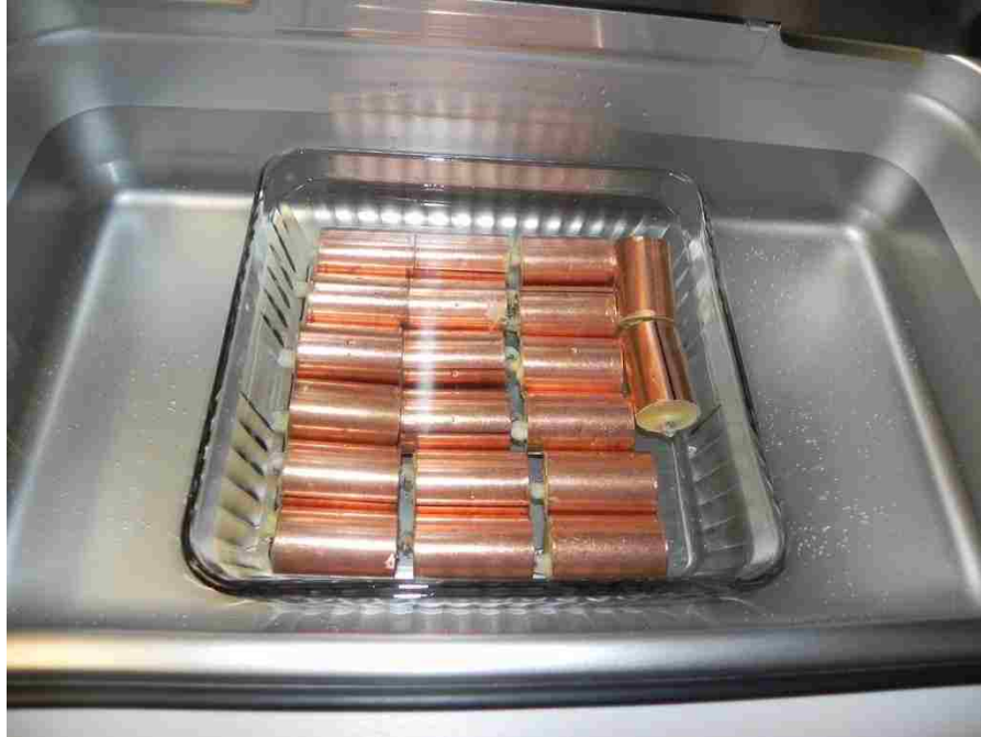
Fig 3.6- Photo of Samples placed into Water Bath: 37 degrees Celsius
