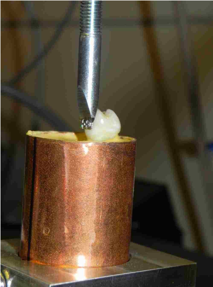
Fig 3.7- Photo of Debonding setup of Universal Testing Machine
