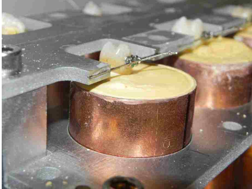
Fig 3.5- Photo of Tooth held in place by Mounting Jig: Tooth secured to wire with steel ligature, held in place by mounting jig
