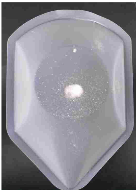
Figure S51: Photograph of the Experiment-9 (100-Mg, Low SiO 2 ) precipitated at 150° C. The precipitate was dried in-vacuo and ground to a fine powder in a mortar and pestle.
