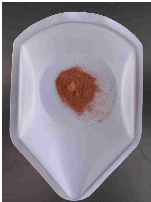
Figure S34: Photograph of the Experiment-4 ( 15\text{-Mg } 85\text{-Fe}^{3+} ) precipitate at 100^\circ\text{C} . The precipitate was dried in-vacuo and ground to a fine powder in a mortar and pestle. Notice the reddish color likely due to the presence of \text{Fe}^{3+} .
