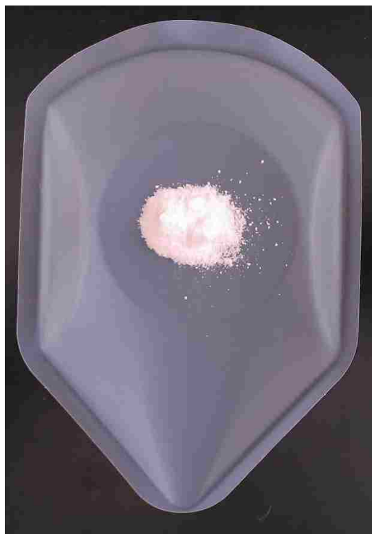
Figure S64: Photograph of the Experiment-12 (50-Al 50-Mg) precipitated at 100° C. The precipitate was dried in-vacuo and ground to a fine powder in a mortar and pestle.
