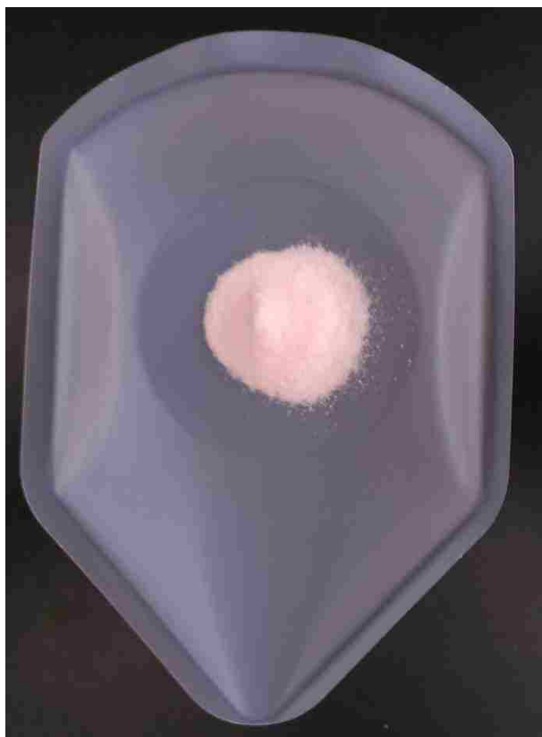
Figure S52: Photograph of the Experiment-9 (100-Mg, Low SiO 2 ) precipitated at 100° C. The precipitate was dried in-vacuo and ground to a fine powder in a mortar and pestle.
