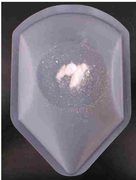
Figure S47: Photograph of the Experiment-8 (100-Al, Low SiO 2 ) precipitated at 150° C. The precipitate was dried in-vacuo and ground to a fine powder in a mortar and pestle.
