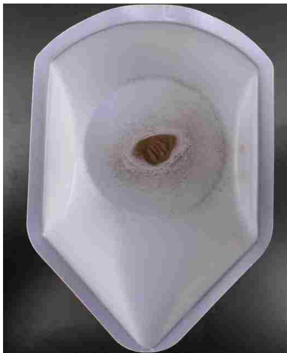
Figure S20: Photograph of the synthetic nontronite control - Experiment-1(100-Fe Control - Subsequently Oxidized) precipitated at 150° C. The precipitate was dried in-vacuo and ground to a fine powder in a mortar and pestle. The reddish color is likely due to the oxidation of the ferrous precursor into nontronite as indicated by our Mössbauer data (Table S3 and S13), as well as the Mössbauer spectroscopy data collected by Mizutani et al. (1991) on material previously produced by this method.
