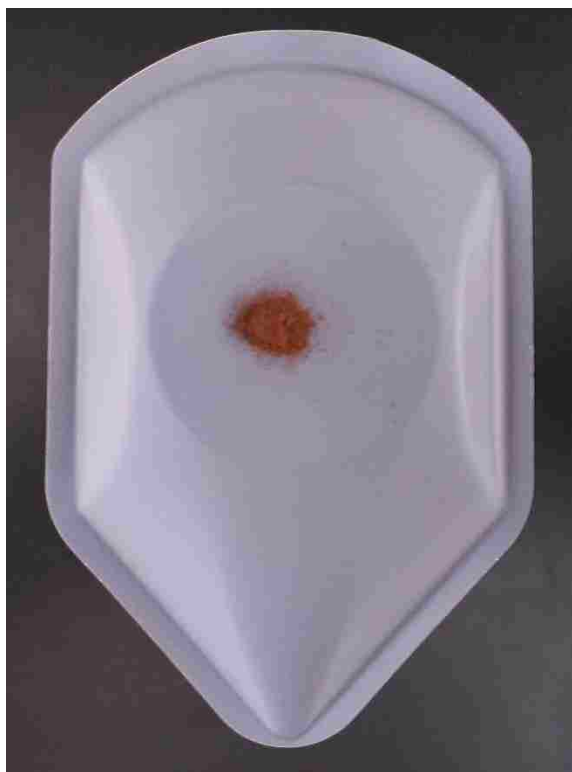
Figure S45: Photograph of the Experiment-7 ( 5\text{-Mg } 95\text{-Fe}^{3+} ) precipitated at 150^\circ\text{C} . The precipitate was dried in-vacuo and ground to a fine powder in a mortar and pestle. Note the reddish color likely from the presence of \text{Fe}^{3+} .
