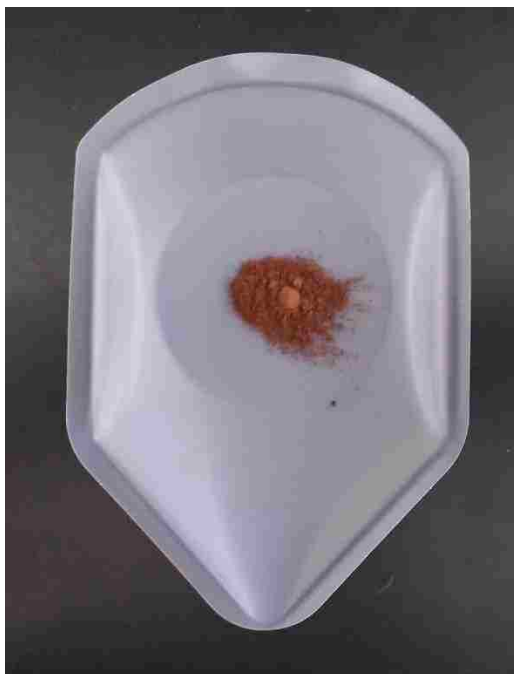
Figure S26: Photograph of the Experiment-2 ( 100\text{-Fe}^{3+} ) precipitated at 100^\circ\text{C} . The precipitate was dried in-vacuo and ground to a fine powder in a mortar and pestle. Notice the reddish color likely from the presence of \text{Fe}^{3+} .
