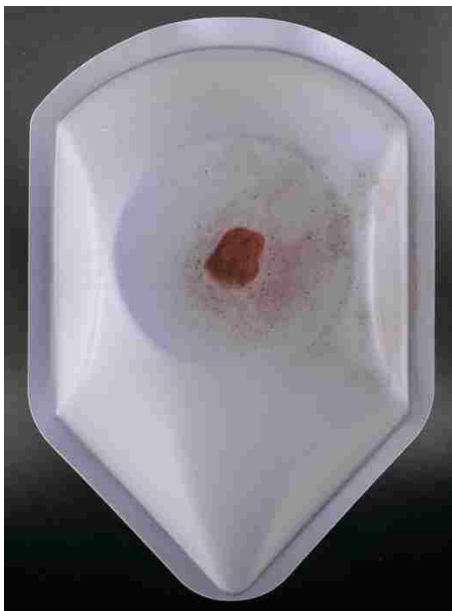
Figure S33: Photograph of the Experiment-4 ( 15\text{-Mg } 85\text{-Fe}^{3+} ) precipitated at 150^\circ\text{C} . The precipitate was dried in-vacuo and ground to a fine powder in a mortar and pestle. Notice the reddish color likely due to the presence of \text{Fe}^{3+} .
