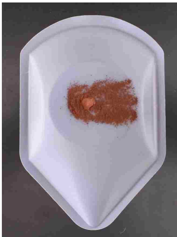
Figure S43: Photograph of the Experiment-6 ( 10\text{-Mg } 90\text{-Fe}^{3+} ) precipitated at 150^\circ\text{C} . The precipitate was dried in-vacuo and ground to a fine powder in a mortar and pestle. Notice the reddish color likely from the presence of \text{Fe}^{3+} .
