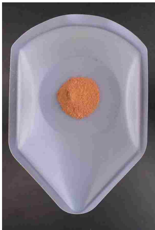
Figure S60: Photograph of the Experiment-11 (44-Al 14-Mg 42-Fe 3+ ) precipitated at 100° C. The precipitate was dried in-vacuo and ground to a fine powder in a mortar and pestle. Note the reddish color likely from the presence of Fe 3+ .
