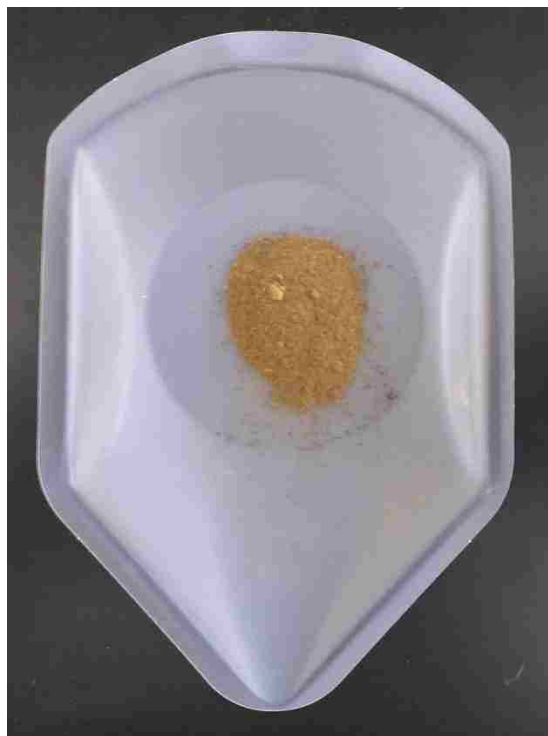
Figure S21: Photograph of the synthetic nontronite control - Experiment-1(100-Fe Control - Subsequently Oxidized) precipitated at 100° C. The precipitate was dried in-vacuo and ground to a fine powder in a mortar and pestle. The reddish color is likely due to the oxidation of the ferrous precursor into nontronite. This is supported by the Mössbauer spectroscopy data collected by Mizutani et al. (1991) on material synthesized in an identical manner, as well as our Mössbauer data of the corresponding 150 ° C experiment (Table S3 and Figure S13).
