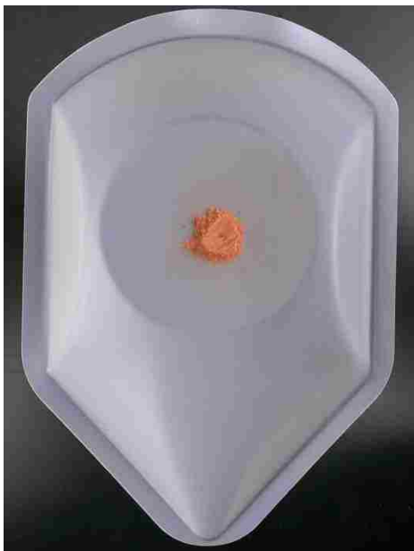
Figure S59: Photograph of the Experiment-11 (44-Al 14-Mg 42-Fe 3+ ) precipitated at 150° C. The precipitate was dried in-vacuo and ground to a fine powder in a mortar and pestle. Note the reddish color likely from the presence of Fe 3+ .
