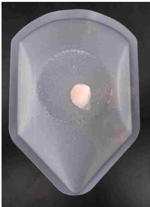
Figure S63: Photograph of the Experiment-12 (50-Al 50-Mg) precipitated at 150° C. The precipitate was dried in-vacuo and ground to a fine powder in a mortar and pestle.
