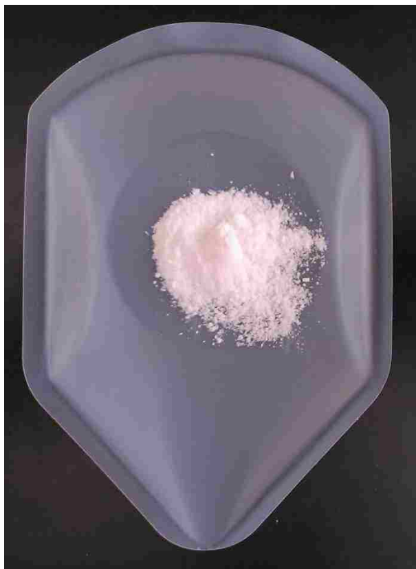
Figure S56: Photograph of the Experiment-10 (100-Al, High SiO 2 ) precipitated at 100° C. The precipitate was dried in-vacuo and ground to a fine powder in a mortar and pestle.
