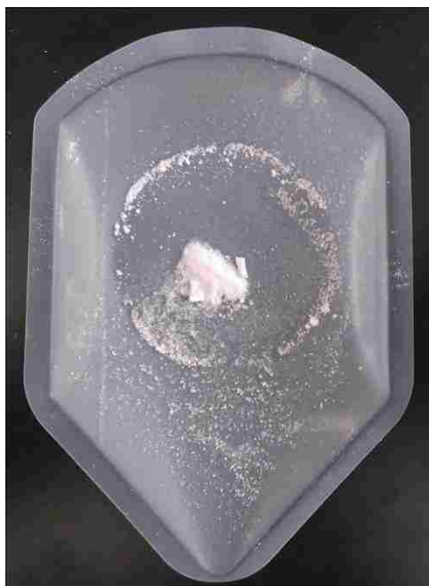
Figure S55: Photograph of the Experiment-10 (100-Al, High SiO 2 ) precipitated at 150° C. The precipitate was dried in-vacuo and ground to a fine powder in a mortar and pestle.
