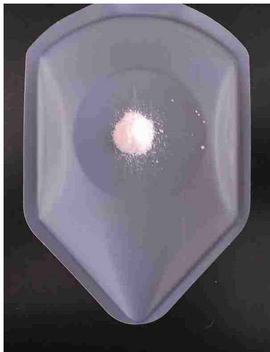
Figure S48: Photograph of the Experiment-8 (100-Al, Low SiO 2 ) precipitated at 100° C. The precipitate was dried in-vacuo and ground to a fine powder in a mortar and pestle.
