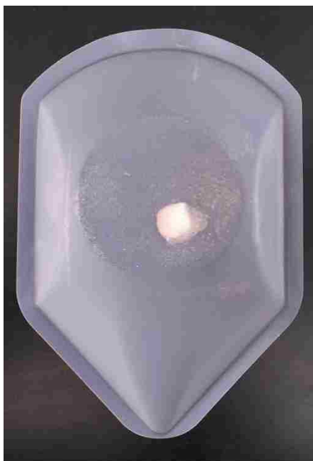
Figure S29: Photograph of Experiment-3 (100-Mg, High SiO 2 ) precipitated at 150° C. The precipitate was dried in-vacuo and ground to a fine powder in a mortar and pestle.
