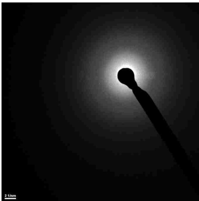
Figure S1: Diffraction pattern from an agglomerate of unaltered synthetic hisingerite, obtained during TEM investigations. Diffuse rings are visible, indicating nanocrystalline structure. Diffractograms were not obtained for synthetic allophane due to its lack of lattice fringes, indicating no long-range order.
