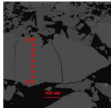
Figure 4.32. Representative EPMA transects across anorthoclase crystals in the Young Rhyolite, along with BSE images of each analyzed crystal with transect plotted in red. Percent Anorthite, Albite, and Orthoclase denoted by symbols.
