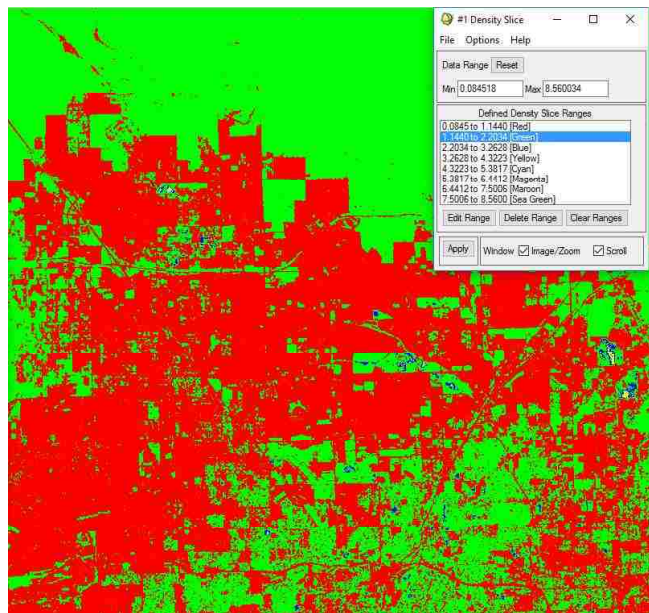
Figure 13: Default density slice overlay in ENVI of Ratio result from Band 5 SWIR 1985/Band 5 SWIR 2010.
