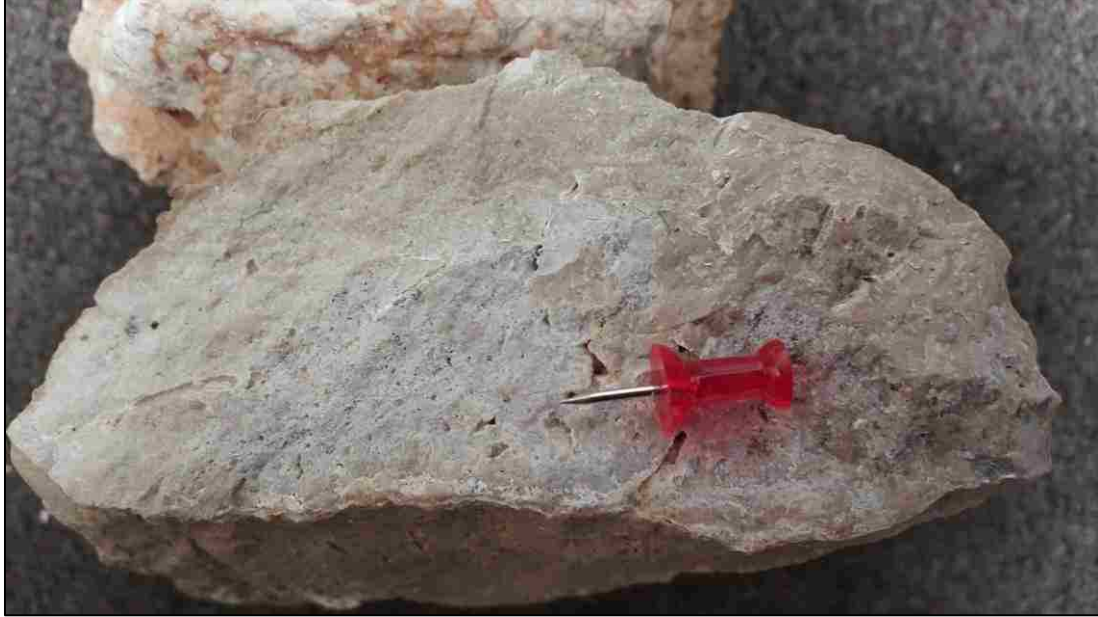
Photo 3. Limestone “b” (Nwlb). The picture shows void-filling calcite that is common in Nwlb.
