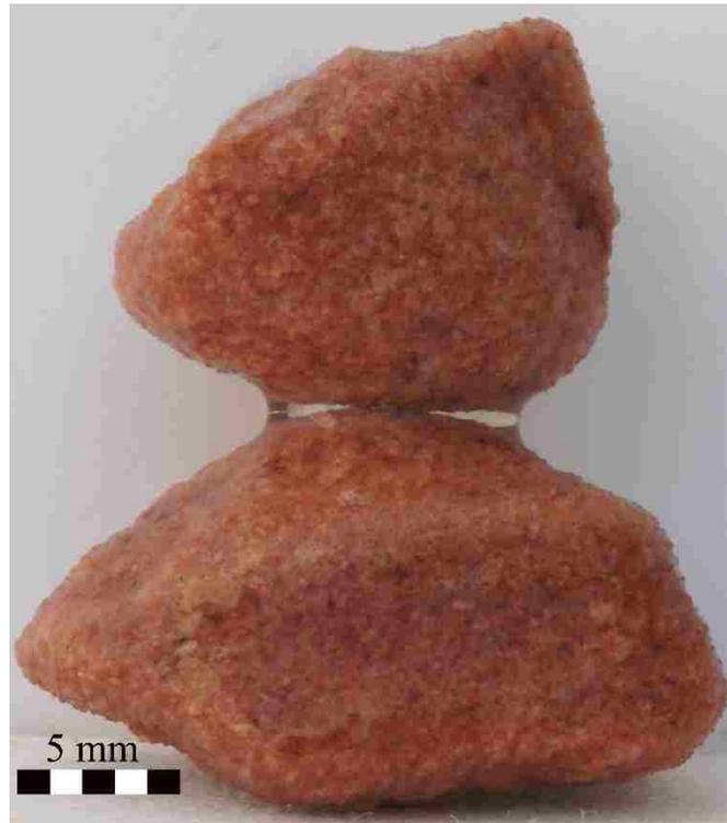
Figure 2.1: A hydraulic bridge connecting two sandstone clasts. Both clasts are rigid and no confining pressure has been applied (negligible deformation at the contact). As a result, the bridge consists primarily of pendular water surrounding a point contact.
