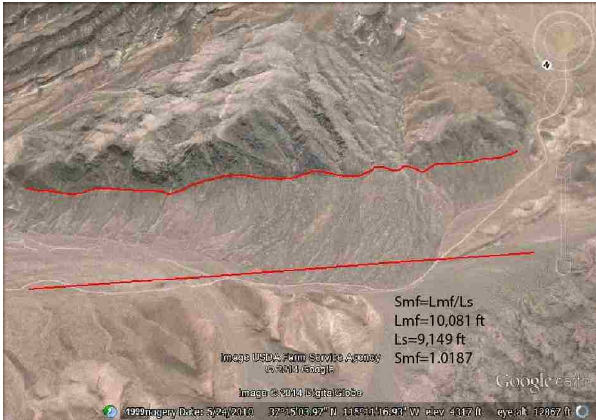
Figure 9. Mountain-front sinuosity showing that the steep hillside side formed recently and may still be active. L_s represents the length of the straight line while L_{MF} represents the length of the mountain front. By dividing the two, the mountain-front sinuosity, S_{mf} , is determined. S_{mf} is a representation of how much the mountain front has eroded since its creation.
