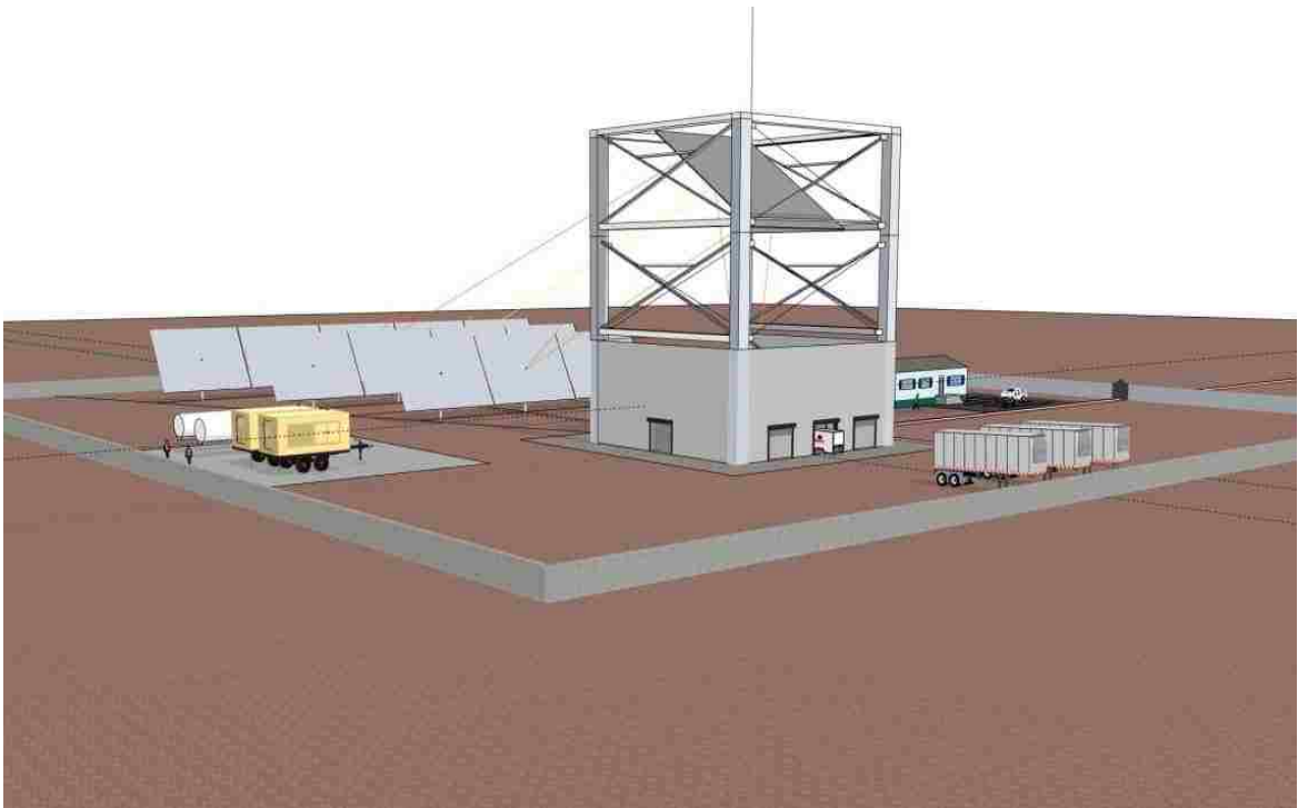
Figure 2.1 NCSETF site layout utilizing temporary infrastructure
