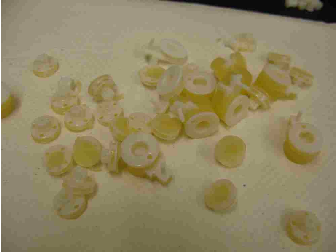
Figure 45: A batch of epicyclic gear arms and gear mounts with support material.
