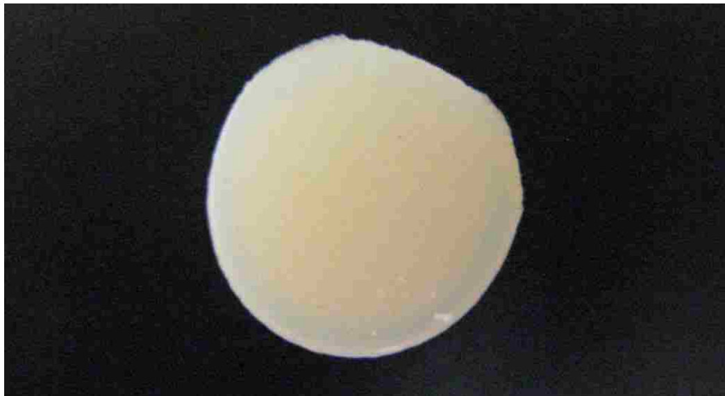
Figure 47: Notice the flat section in the upper right corner. This should be a perfect circle.
