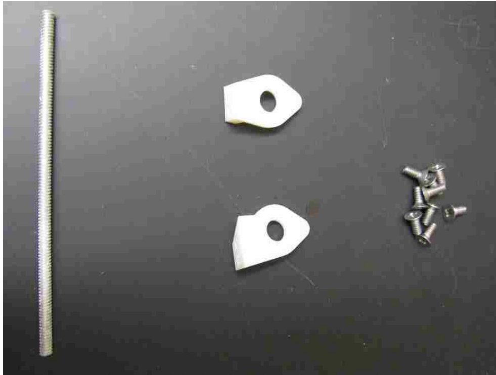
Figure 39: ANSI#8-32 aluminum threaded rod used in the linear actuator, fasteners for the stepper motors, and screws used to attach the fasteners.
