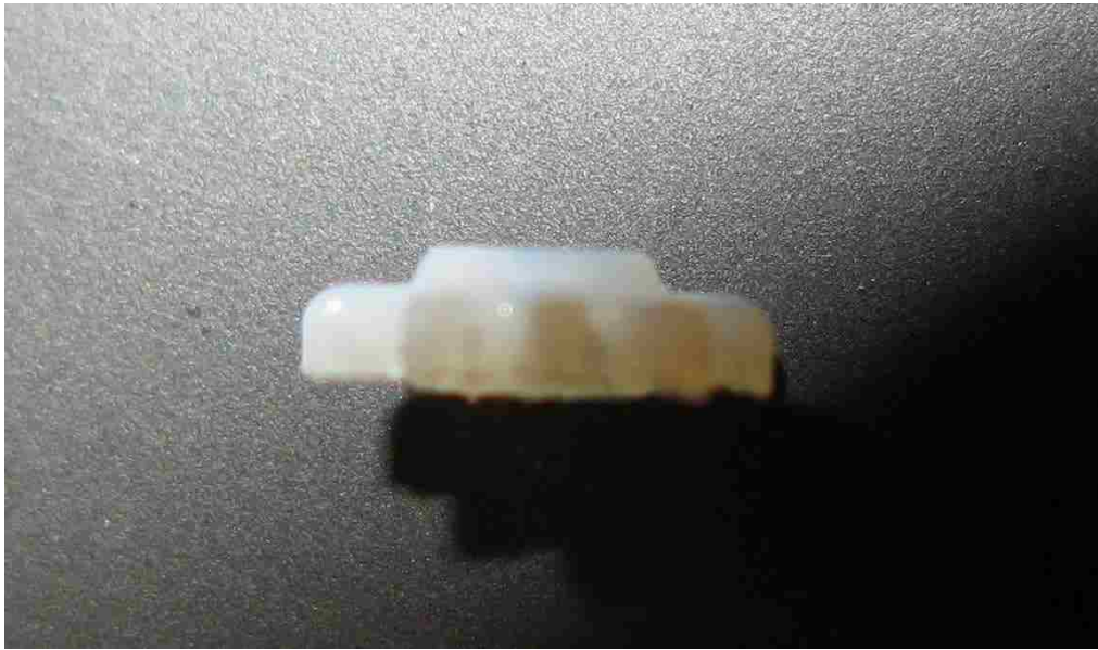
Figure 46: This spur gear should be symmetric through a roughly horizontal line, but the burr on the bottom makes this obviously not so.
