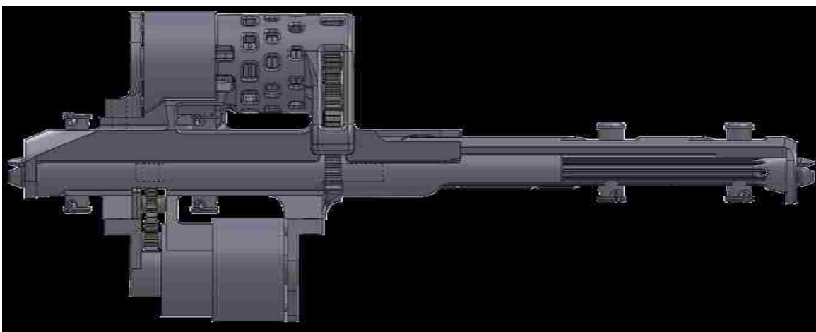
Figure 36: One full link of the prototyped mechanism with a rotary and prismatic actuator. Because all links are the same, one link might be considered to be a more fundamental module than the triangular module adopted for this project.
