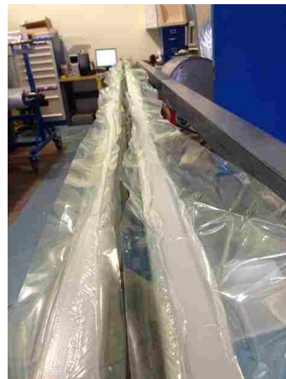
Figure 8: Vacuum bag covering aluminum extrusion of inner half
