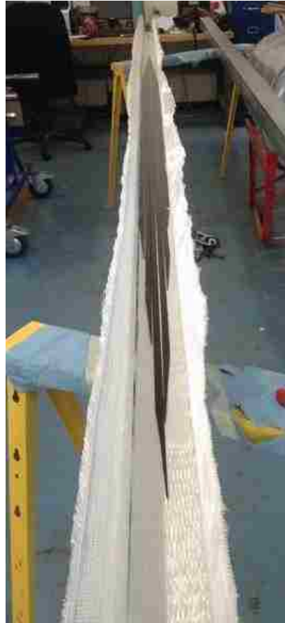
Figure 9: Layup of carbon fiber pultrusions on flange for inner half
