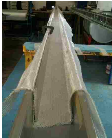
Figure 5: Layer of DB240( \pm 45^\circ ) on aluminum extrusion for inner half
