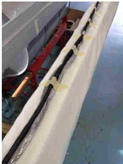
Figure 7: Peel Ply and distribution medium on aluminum extrusion for outer half
