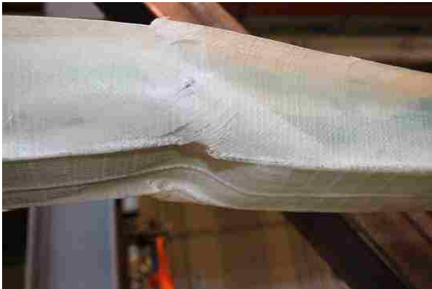
Figure 11: Buckling in webs and deformed compression flange
