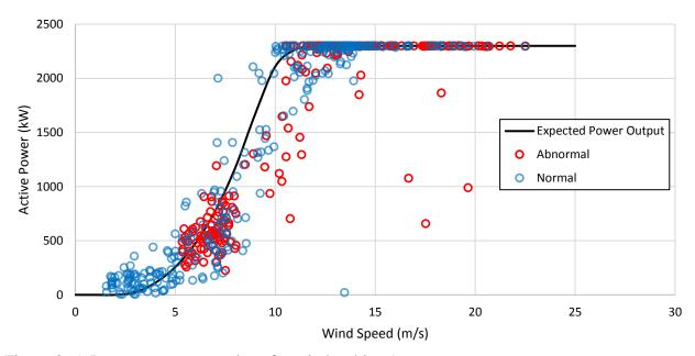
Figure 3. 5: Power curve comparison for wind turbine 1.
