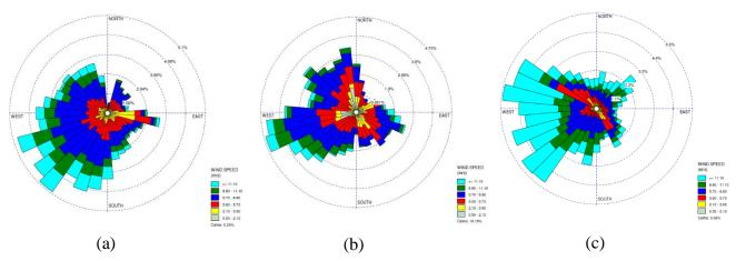
Figure 2. 2: Wind rose for (a) wind farm 1, (b) wind farm 2, and (c) wind farm 3 measured by on-site meteorological mast.
