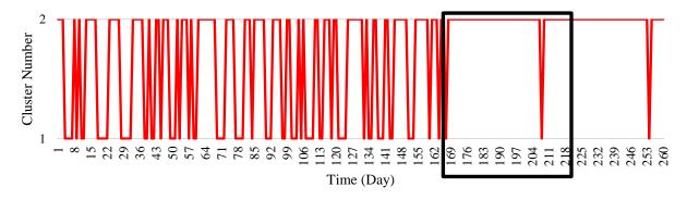
Figure 4. 5: Assigned clusters for each day for the first 260 days of the dataset for wind turbine 42 with a 50-day moving window.
