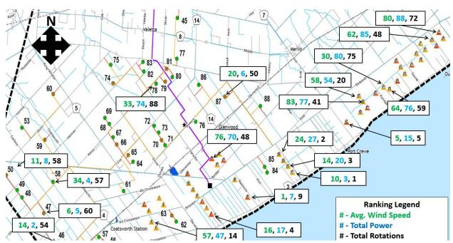
Figure 2. 3: Ranking of wind speed and select SCADA variables (from highest to lowest) for select turbines at farm 1.
