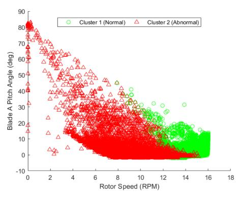
Figure 4. 1: Clustering results from monitoring blade SCADA parameters with rotor speed and blade pitch shown.
