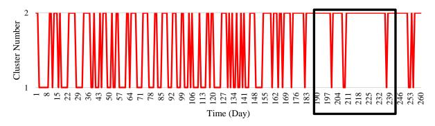
Figure 4. 6: Assigned clusters for each day for the first 260 days of the dataset for wind turbine 47 with a 50-day moving window.
