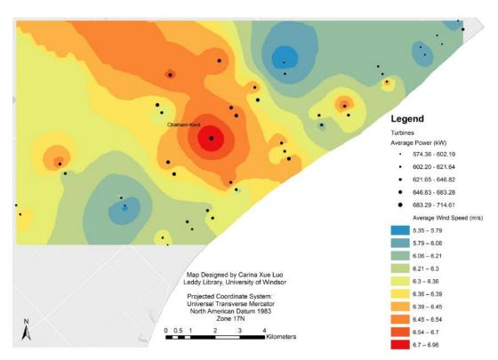
Figure 2. 5: Average wind speed and average power produced for wind farm 2.
