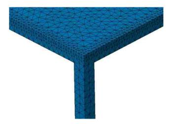
Figure 4.8 A zoomed view of the local mesh of the solid Catia FE model of the platform under harmonic response
