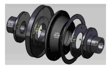
Figure 1.46 The Periflex coupling studied, exploded view [13]
