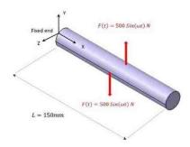
Figure 3.10 Fully 3D Model of the Fixed-Free beam under a harmonic moment at the middle point
