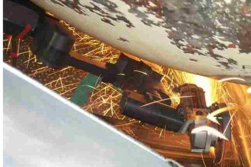
Figure 1.52 SCOMPI robot developed by Research Institute of Hydro-Quebec [16]
