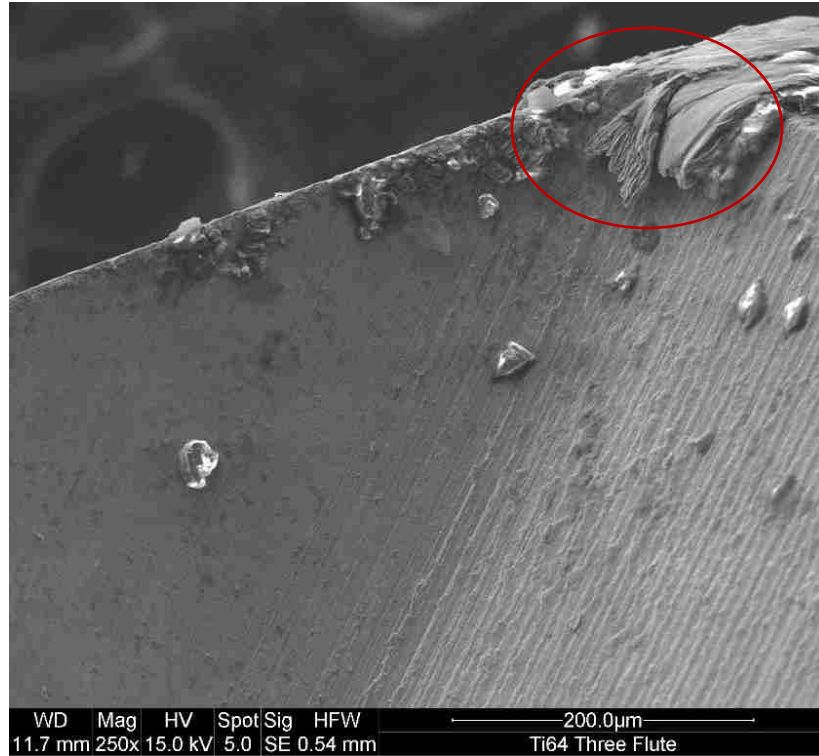
Figure 76. 250x SEM flute view of the three flute drill bit cutting edge after drilling 60 holes in grade 5 titanium (Ti-6Al-4V).
