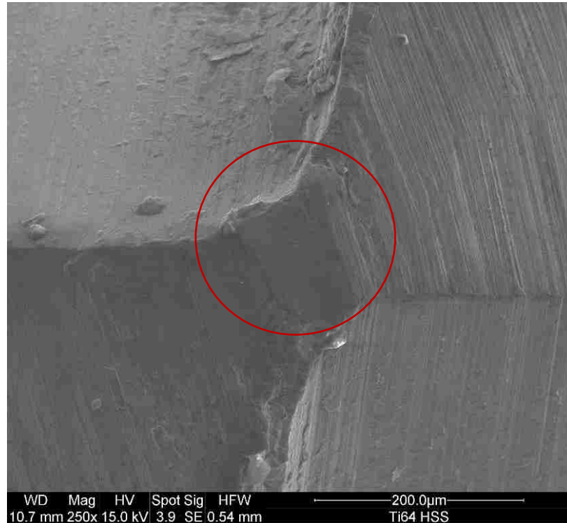
Figure 41. 250x SEM view of the HSS drill bit chisel edge after drilling 60 holes in grade 5 titanium (Ti-6Al-4V).
