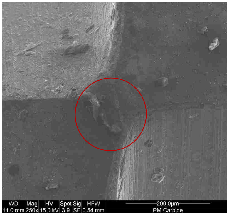
Figure 111. 250x SEM top down view of the chisel edge of the carbide drill bit after drilling 60 holes in PM titanium.
