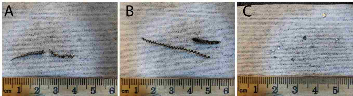
Figure 166. Chip morphology after drilling (A) grade 5 titanium (Ti-6Al-4V) for 60 holes, (B) PM titanium for 60 holes, and (C) AM titanium for 23 holes using a three flute drill bit.
