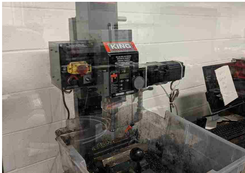
Figure 39. Drilling setup showing the CNC drill press and computer.
