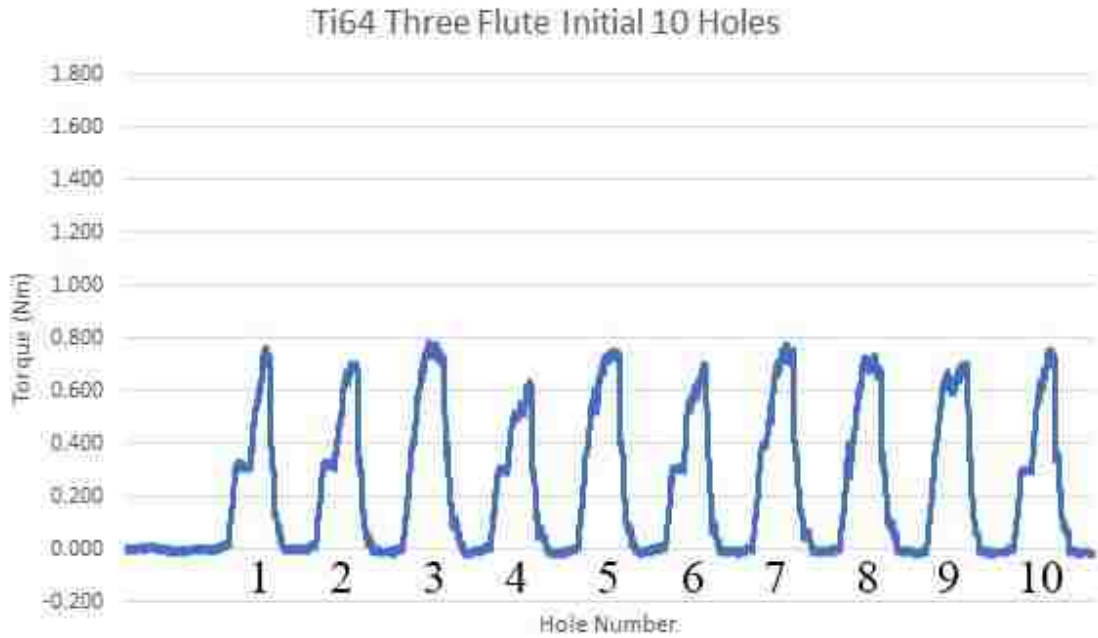
Figure 140. Torque data for the initial 10 holes when drilling 60 holes in grade 5 titanium (Ti-6Al-4V) with the three flute drill bit.
