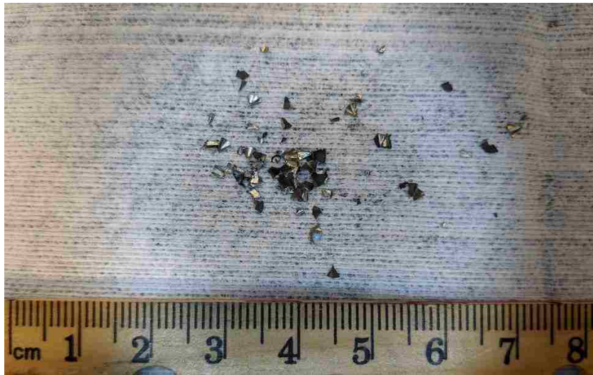
Figure 165. Chip morphology of AM titanium using an HSS drill bit after drilling and failing at 8 holes.
