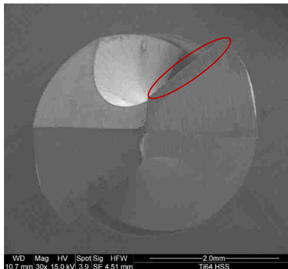
Figure 40. 30x SEM top down view of the HSS drill bit after drilling 60 holes in grade 5 titanium (Ti-6Al-4V).
