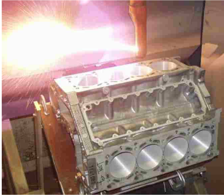
Figure 1.4 PTWA coating of the bores of a BMW M62 gasoline engine [71].
