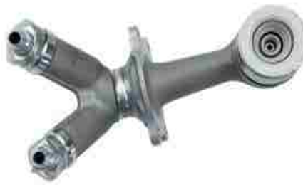
Figure 1. 1 3D printed fuel Nozzle tip for LEAP engine [1]
