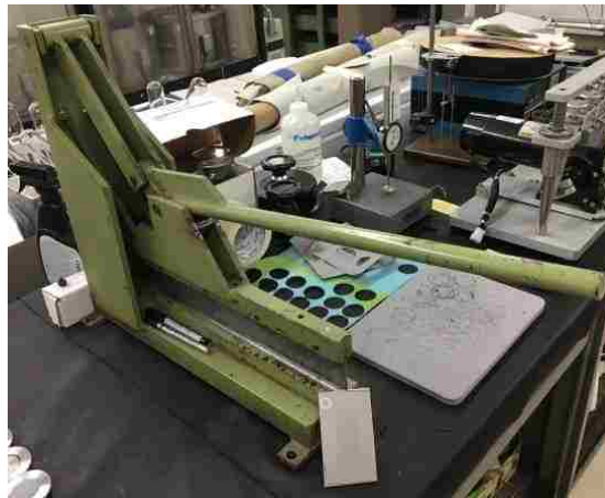
Figure 42. Cutter for specimens preparation.
