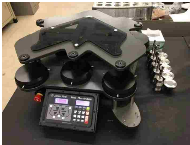
Figure 43. Martindale Abrasion Tester.
