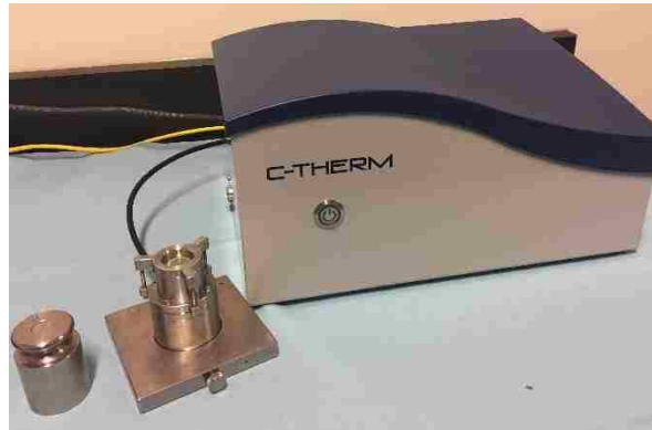
Figure 5.2 Thermal conductivity analyzer device (C-therm)
