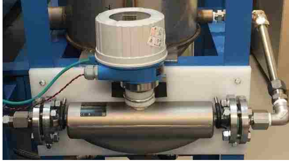
Figure 2.6 Mass flow meter (Coriolis technology)
