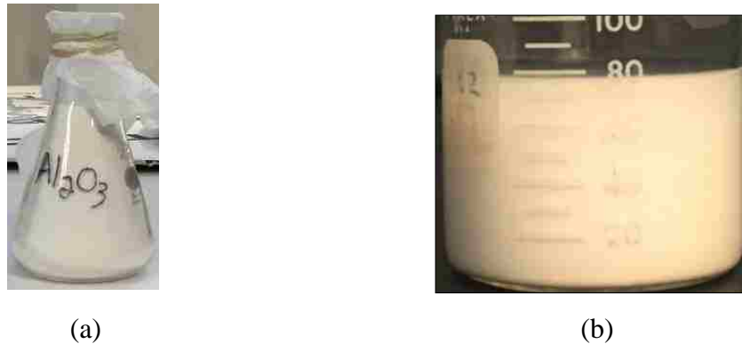
Figure 5.1 samples of (a) Al_2O_3 nanoparticles (50nm) and (b) Al_2O_3/W nanofluid (volumetric concentration = 5%)
