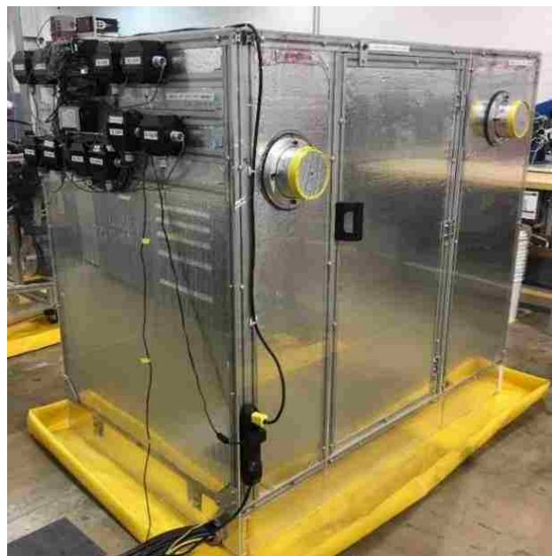
Figure 3. 31 – Port holes on insulated chamber for cold testing.
