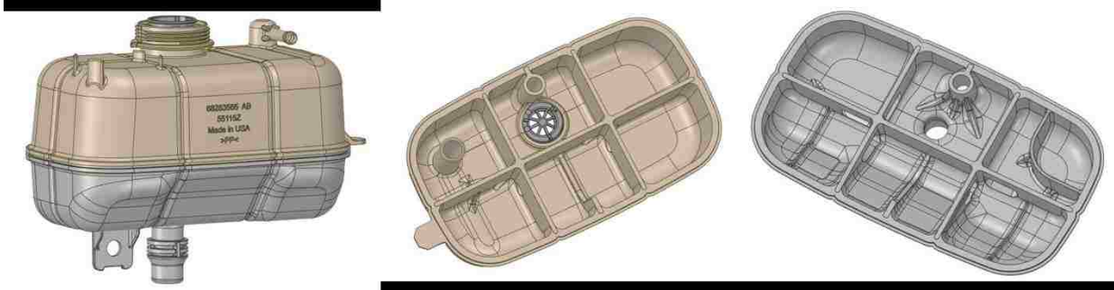
Figure 4.11 – Dissected bottle CAD for detailed geometry investigation.
