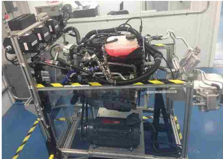
Figure 3. 2 – Side view of engine cooling system flow bench.
