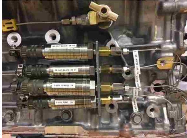
Figure 3. 28 – Water jacket instrumentation cluster mounted on engine exterior.
