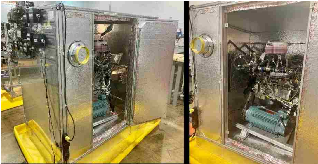
Figure 3. 29 – Insulated system level bench chamber.
