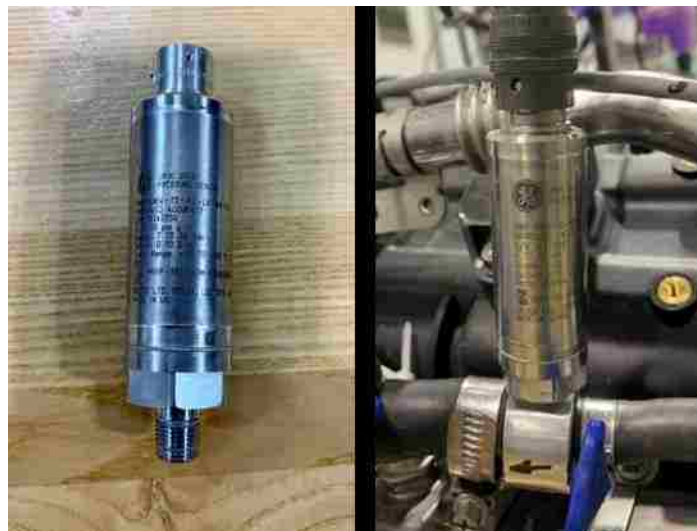
Figure 3. 3 – Pressure sensor, before and after bench installation.
