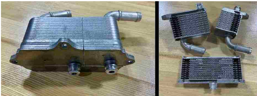
Figure 4. 5 – Dissected TOH for detailed geometry investigation.
