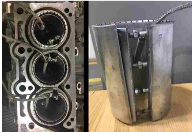
Figure 3. 30 – Engine block cylinder bore heaters.
