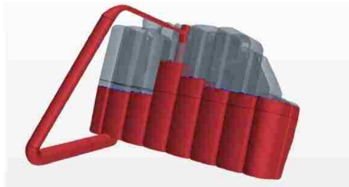
Figure 2. 5 – Hot bottle internal coolant distribution [10].
