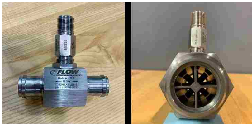
Figure 3. 4 – Flow meter, front and cross-section views.
