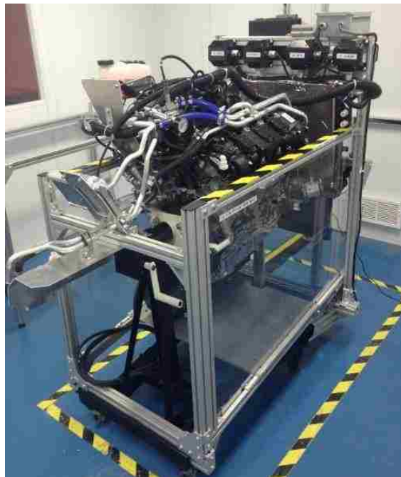
Figure 3. 1 – Isometric view of engine cooling system flow bench.
