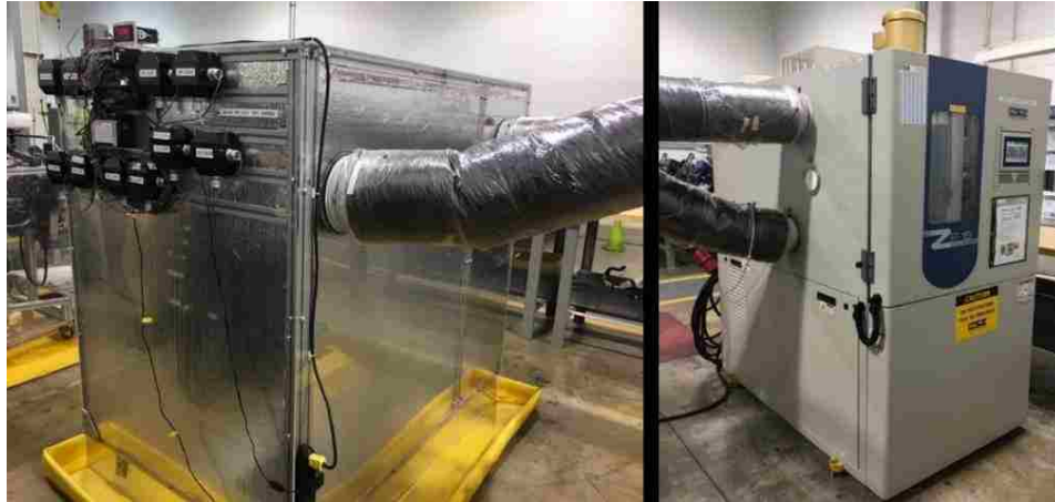
Figure 3. 32 – Remote conditioning unit fitted to insulated chamber.
