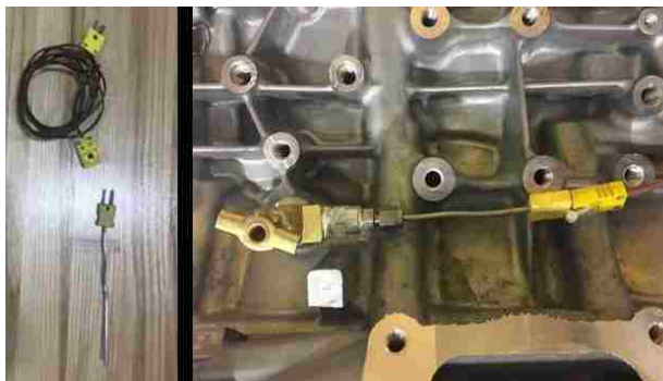
Figure 3. 5 – Thermocouple, before and after bench installation.
