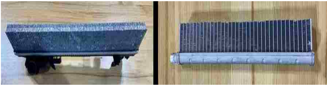
Figure 4. 2 – Dissected radiator and heater core for detailed geometry investigation.
