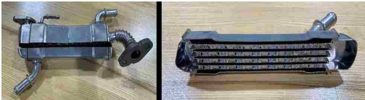
Figure 4. 8 – Dissected EGRc for detailed geometry investigation.
