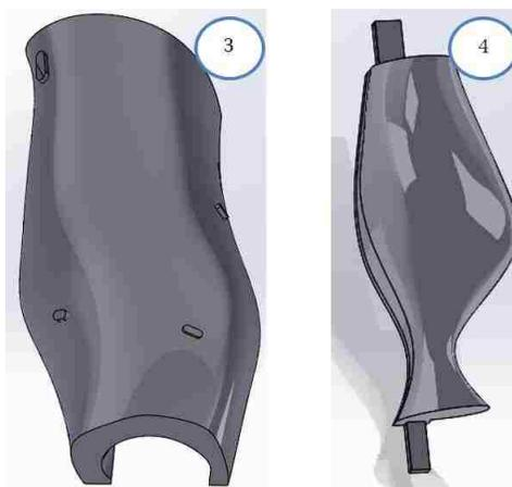
Figure 4.4-2 (a): Tissue spacer insert, (b): Inner thoracic cavity mould
