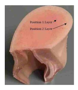
Figure 4.6.1-2: Dual layer composition of alpha prototype
