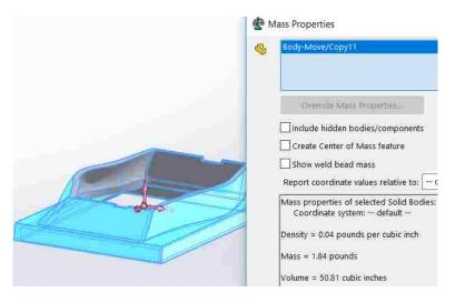
Figure 3.3.2-6: Measurement of mass properties of mould top
