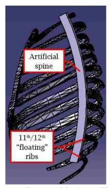
Figure 3.1-4: Rib cage model spine modifications
