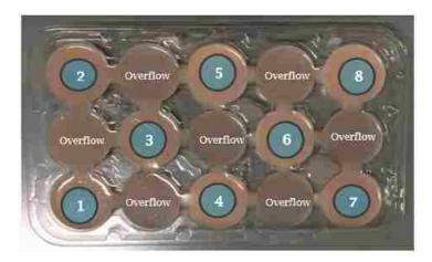
Figure 3.4-1: Isolated silicone layers with varying constitutions
