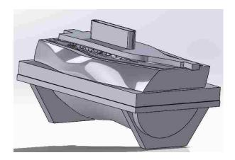
Figure 4.4-6: Completed, assembled optimized mould set
