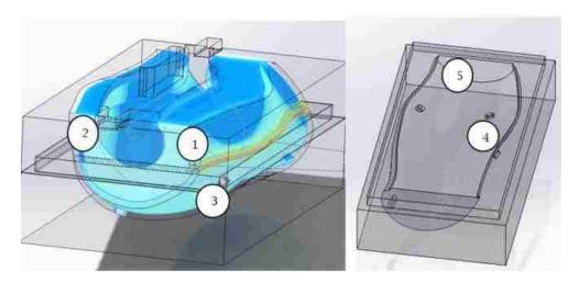
Figure 3.3.1-1: Quick-change mould modifications
