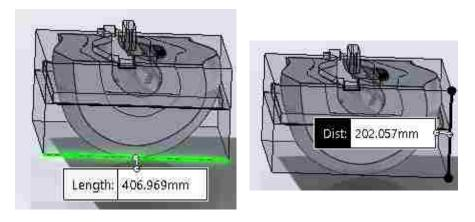
Figure 3.3-5 (a) and (b): Dimensions of intiial mould block configuration
