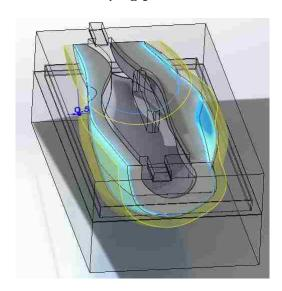
Figure 3.3-3: Parametric offset of tissue and mould
