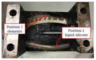
Figure 4.6.3-2: Position 1 silicone pouring set-up (weights included in image are for holding down the hollow—and therefore buoyant mould inserts)
