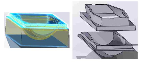
Figure 3.3.2-2 (a): "Thickening" of mould faces to obtain solid body, (b): Upper and lower thickened mould elements
