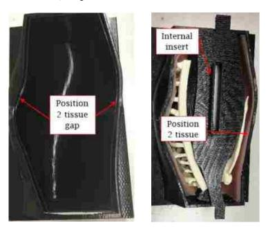
Figure 3.5.1-1 (a): Mould set gap for pouring of first silicone layer, (b) Preparation for second silicone pour of two-pour overmoulding procedure
