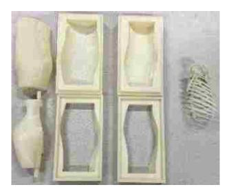
Figure 4.5-5: Quick-change mould elements
