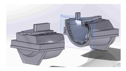
Figure 3.3.2-5 Split mould set for fabrication using smaller build envelopes
