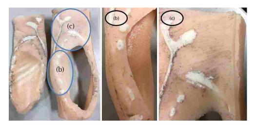
Figure 4.6.2-1: Cross sectional analysis of silicone prototype
