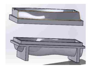
Figure 3.3.2-3: Mould base supports
