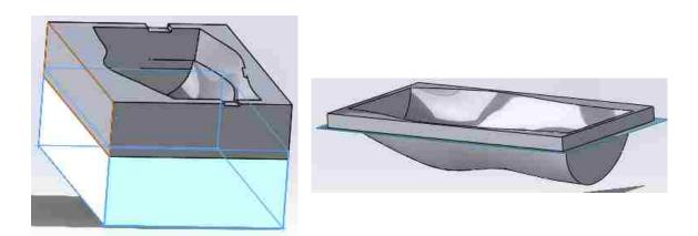
Figure 3.3.2-1 (a): Deletion of perimeter faces, (b) Remaining inner and upper surfaces of mould base
