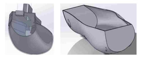
Figure 3.3.2-4: "Shelled" artificial tissue and mould insert
