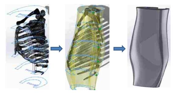
Figure 3.3-1: Spline lofting for artificial tissue representation
