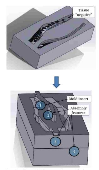
Figure 3.3-2 (a): Tissue 'negative" (top), (b): Insert and assembly feature modifications (bottom)
