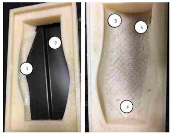
Figure 4.5-6: Key quick-change mould element features
