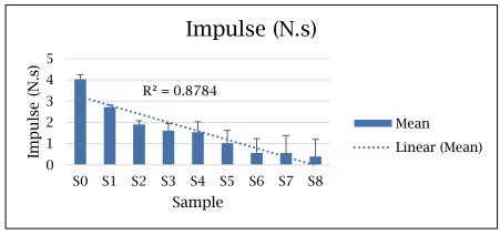
Figure 4.3.1-2: Impulse means for silicone sample needle insertions
