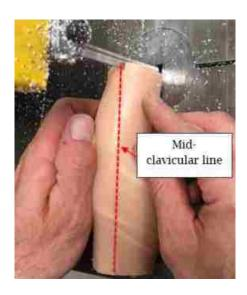
Figure 3.5.1-3: Cross-sectional analysis preparation of simulated thoracic wall representation
