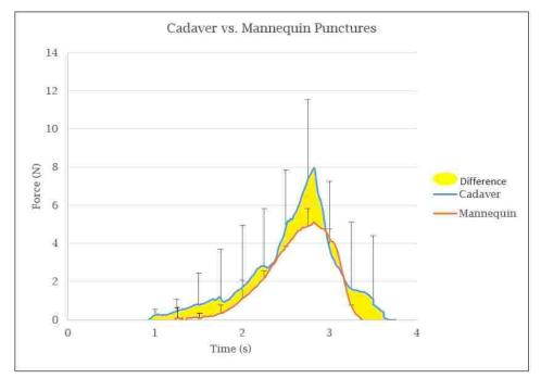
Figure 4.2.1-7: Manually processed position 3 cadaver and THM-30 simulator puncture curves
