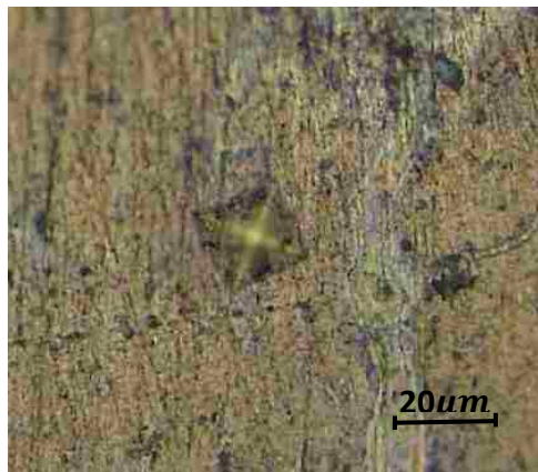
Figure 4-4: Micro-Vickers indentation on the AA5754-O skin with typical square indentation and diagonals.
