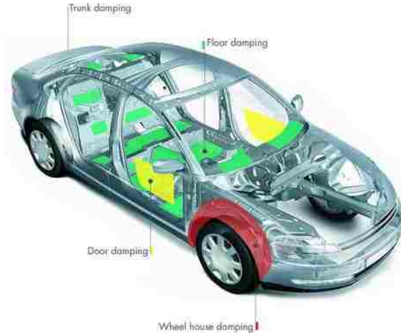
Figure 1-4: Damping patches location in the vehicle [6].
