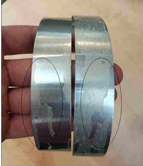
Figure 4-33: Quiet Aluminum® strips with AA5754-O skin in the as-received condition. The image shows the inner surfaces of the sandwich after T-peel test. The specimen presented adhesive failure mode. The black circles are examples of the polymer attached to one surface and the other in a complementary way.
