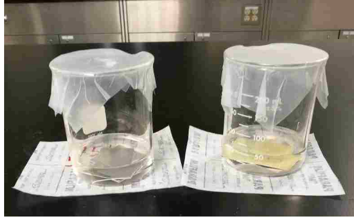
Figure 3-10: Roughness specimens submerged into acetone to dissolve the polymer core.
