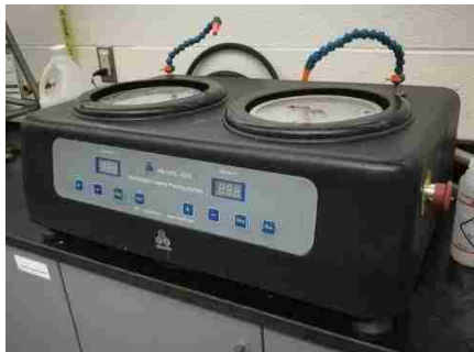
Figure 3-4: UN I POL – 820 Metallographic Lapping /Polishing Machine available at the University of Windsor.
