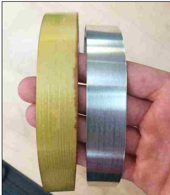
Figure 4-32: Quiet Aluminum® strips with 6061-T4 skin after the hardening procedure (1 h at 200°C). The image shows the inner surfaces of the sandwich strip after T-peel test. The specimen presented adhesive failure mode, with the polymer completely attached to one surface. Degradation of the polymer could be observed due to burning.
