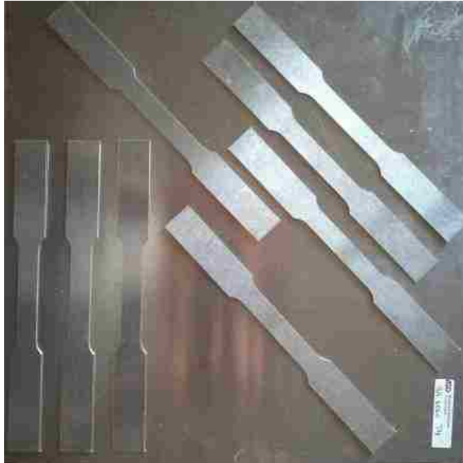
Figure 3-9: Specimens cut with water jet technology.
