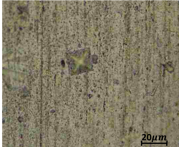
Figure 4-5: Micro-Vickers indentation on the AA6061-T4 skin with typical square indentation and diagonals.
