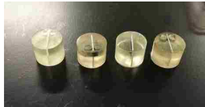
Figure 3-3: Samples were mounted in epoxy for cross-sectional view.
