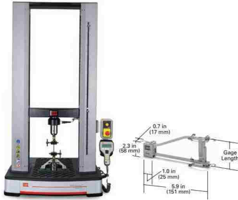
Figure 3-5: MTS Model 43 Universal Tensile Testing Machine and MTS Axial Extensometer 50 mm gauge length [44].
