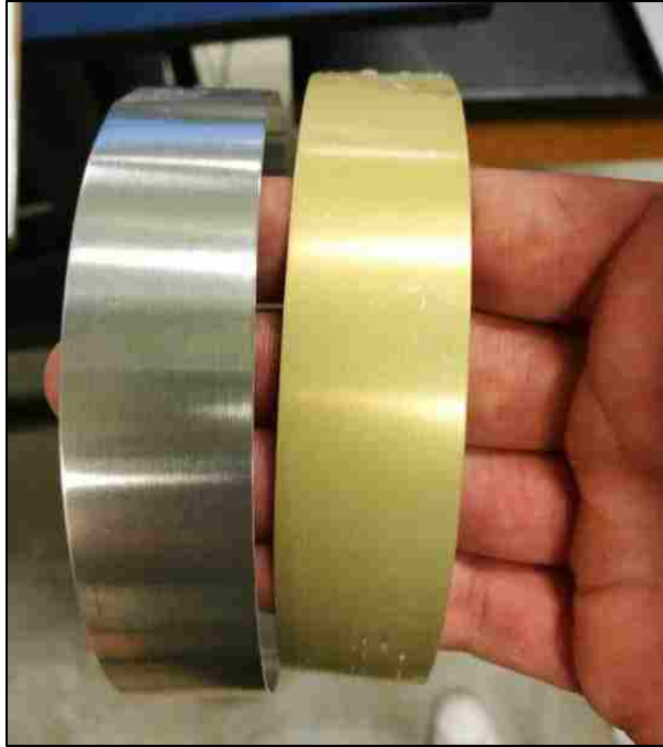
Figure 4-31: Quiet Aluminum® strips with 6061-T4 skin in the as-received condition. The image shows the two inner surfaces of the sandwich strip after T-peel test. The specimen presented adhesive failure mode, with the polymer completely attached to one surface.
