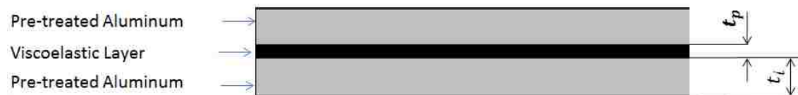
Figure 3-1: Schematization of the sandwich structure. The thickness t_i is approximately 0.5 \text{ mm} , whereas t_p is approximately 0.03 \text{ mm} . [8]
