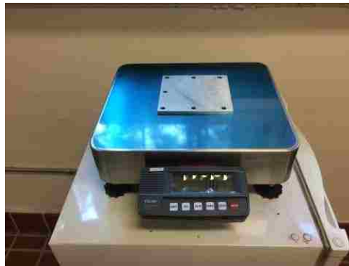
Figure 28: Scale used to weigh the filter.
