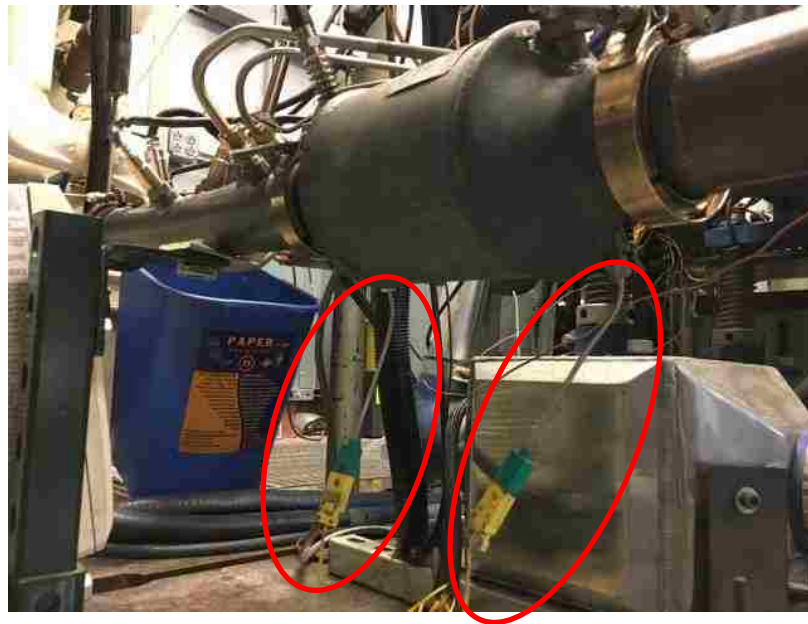
Figure 27: Thermocouples applied on the GPF.
