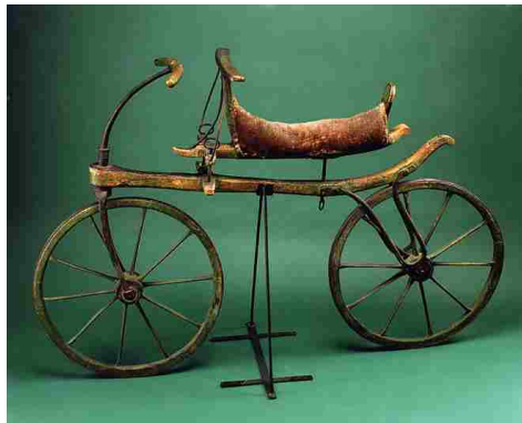
Figure 1.3: The draisine, or running machine (reproduced from Smithsonian National Museum[8])
