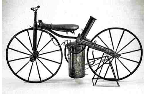
Figure 1.7: Sylvester Roper steam motorcycle. (reproduced from The Smithsonian Museum[25])
