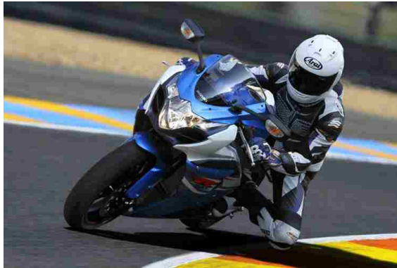
Figure 1.10: Suzuki ® GSX-R1000. This motorcycle has a maximum output power of approximately 117 kW at 13200 rev/min. The corresponding top speed is in excess of 80 m/s [288 km/h]. (reproduced from contramanillar.com [tr. countermeasures.com ][28])
