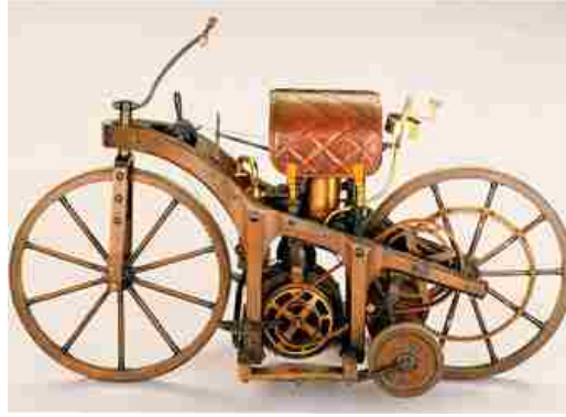
Figure 1.8: Daimler petrol-powered motorcycle. (reproduced from The American Society of Mechanical Engineers[26])
