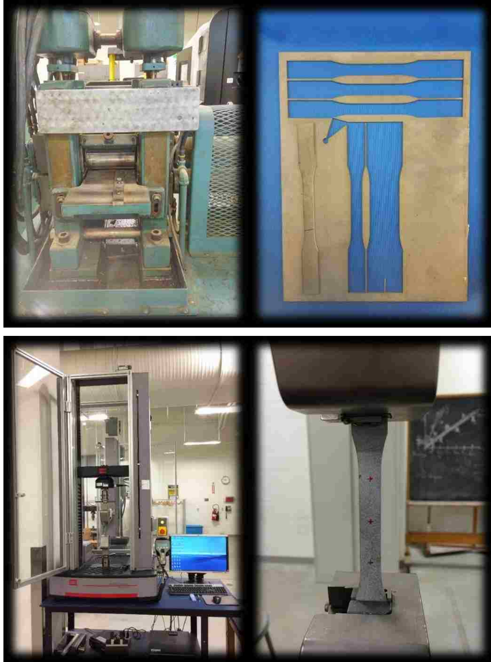
Figure 58 – the Flat Roller, the EDM tensile specimen and the tensile test setup
