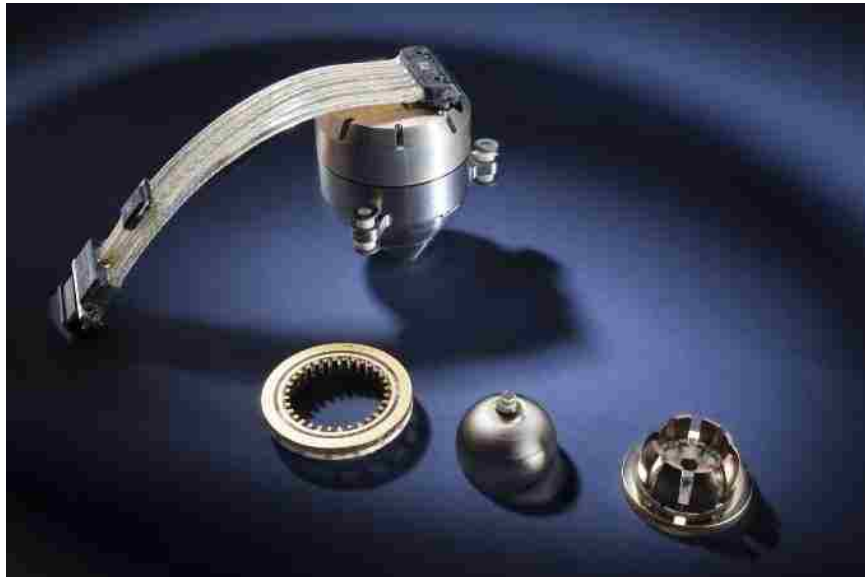
Figure 2: Hemispherical resonator gyro and its components [18]
