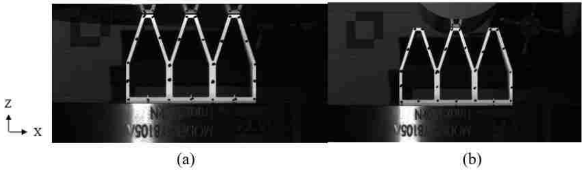
Figure 27. Test setup of (a) flat platter compression, (b) roller compression.
