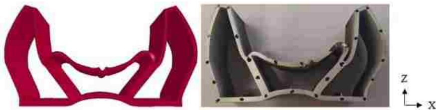
Figure 32. Deformed shape after roller compression.
