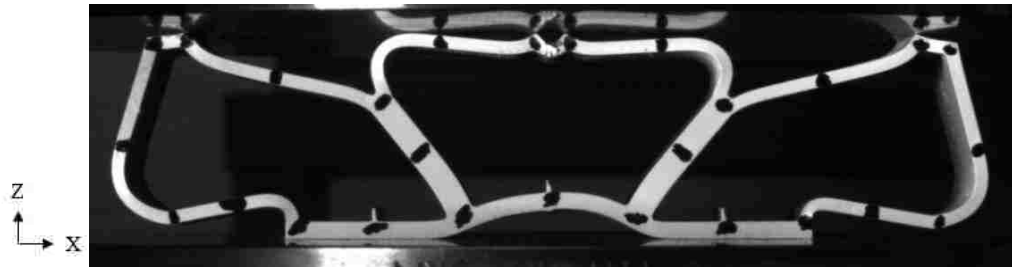
Figure 37. Deformed specimen at 17 mm of flat platter compression.
