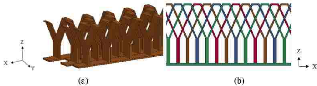
Figure 40. Finite element model of revised structure: (a) section of structure with symmetrical cut-off and (b) layers of structure differed with color.
